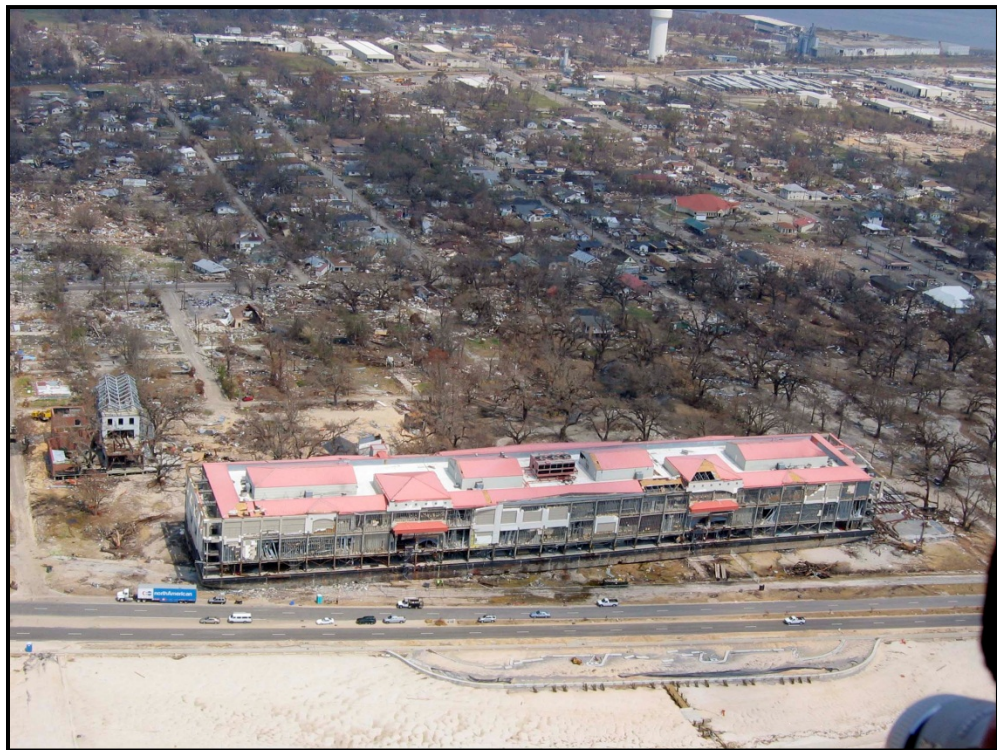
Figure 33. Grant Casino in Biloxi after Hurricane Katrina. It broke free of its moorings and landed on top of the National Register-listed Tullis-Toledano House. Source: FEMA.
