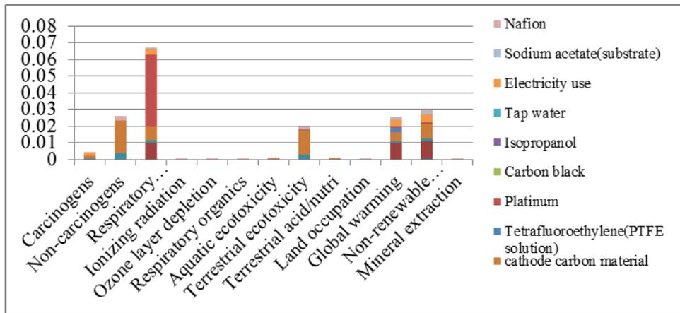
Figure 11: Normalized side-lying design MFC environmental impact per midpoint category (hybrid method result)
