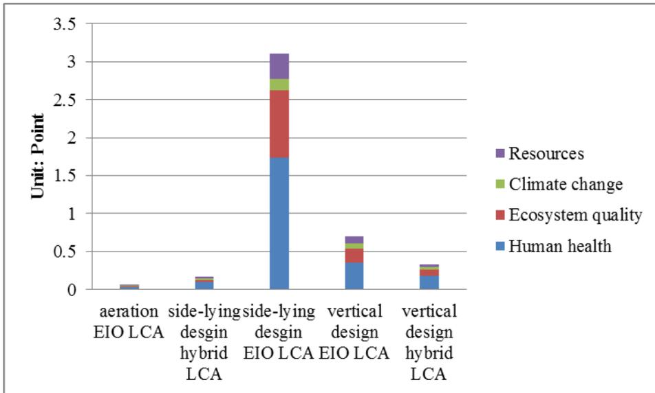
Figure 12: Environmental impact comparison of MFC systems with aeration system
