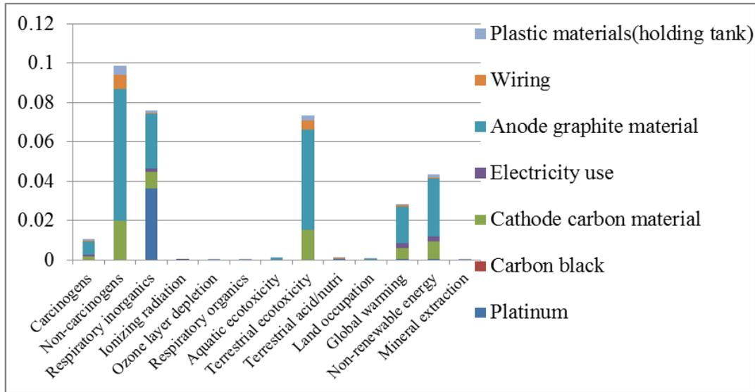
Figure 8: Normalized vertical design MFC environmental impact per midpoint category (hybrid method result)
