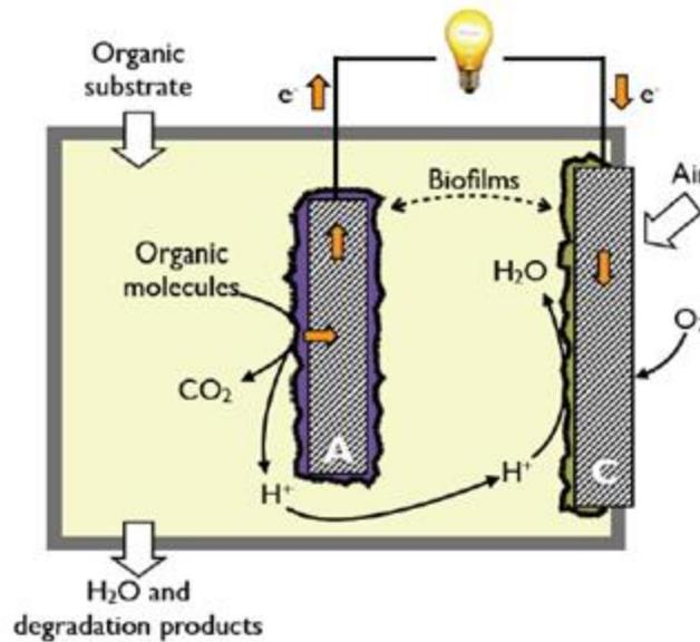
Figure 2: Schematic diagram of a single-chamber MFC((Degrenne et al., 2011))
