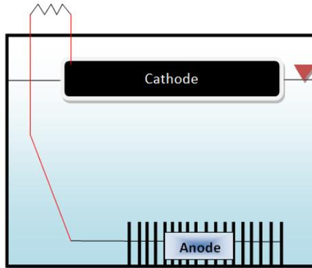
Figure 4: Schematic diagram of vertical design MFC
