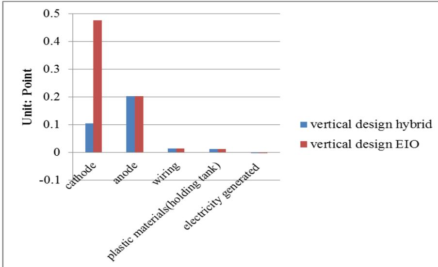
Figure 7: Vertical design MFC overall environmental impact per component (EIO method and hybrid method result)
