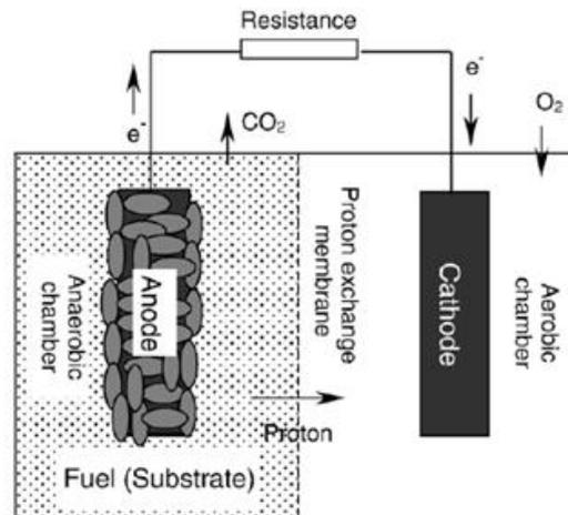
Figure 1: Schematic diagram of a two-chamber MFC (Du et al., 2007)
