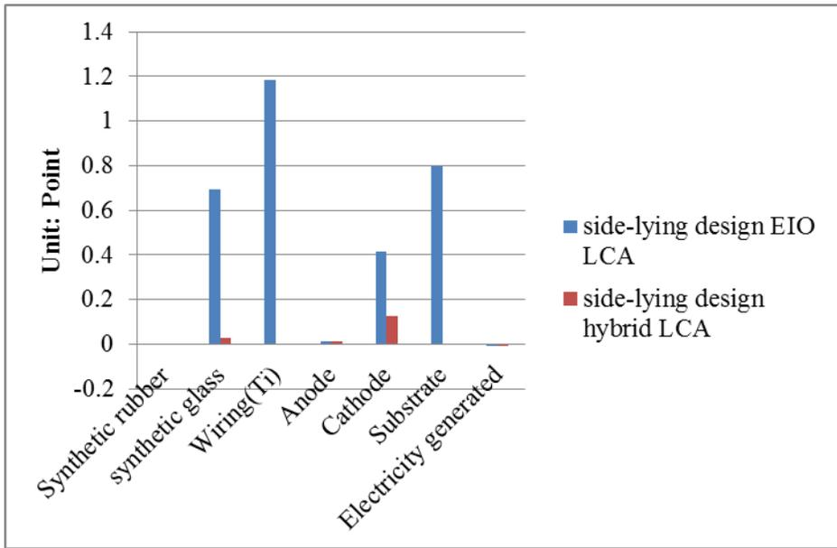
Figure 10: Side-lying design MFC overall environmental impact per component (EIO LCA and hybrid method result)
