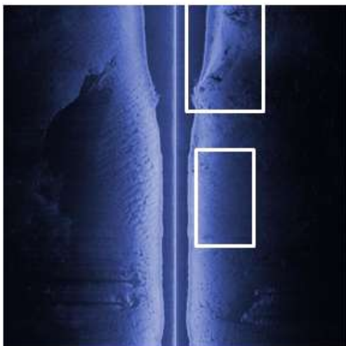
Gravel – Dimpled texture, strong return, larger (10cm) pieces of rock may be observable.
