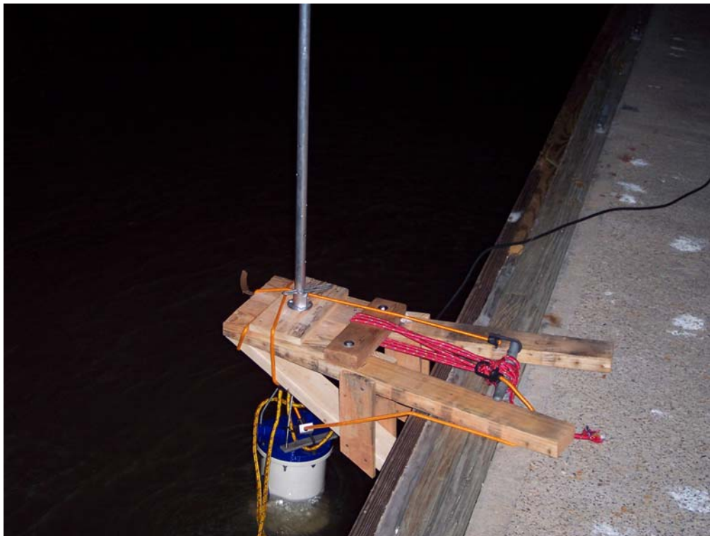
Fig. 12. Tethered ADCP on floating dock.
