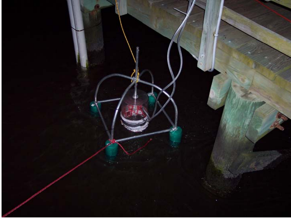
Fig. 10. Floating chamber tethered from front to prevent movement under dock. This is an example of a high current speed deployment.
