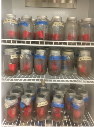
Figure 3.3. Soil incubation chamber filled with glass jars.
