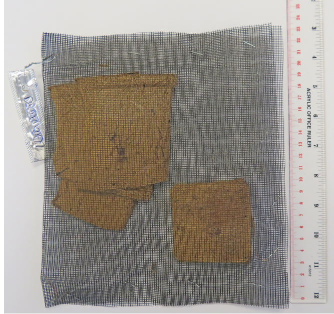
Figure 2.2. Mesh litter bag with aluminum label containing biodegradable container (15.25 cm x 25.4 cm, 0.02 cm mesh diameter)
