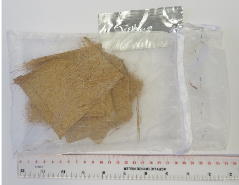
Figure 2.4. Organza mesh litter bag containing biodegradable container (12.7 cm x 17.8 cm, 0.01 cm mesh diameter).
