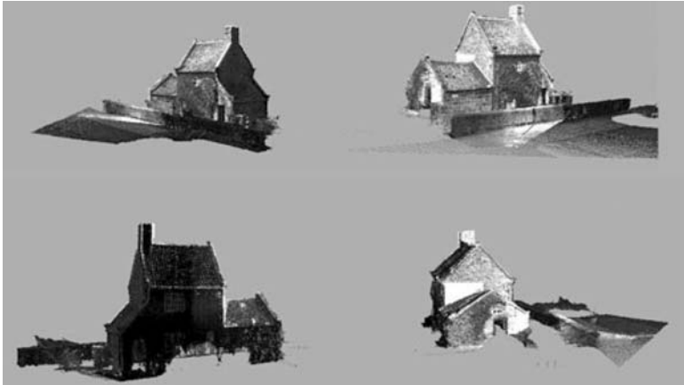
Figure 4.7. The 3D point cloud resulting from the combination of the data sets from the four scans. 72
