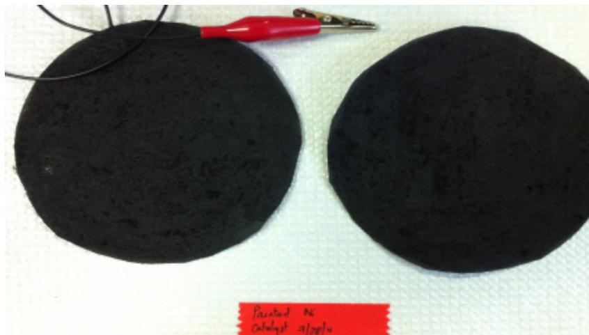
Figure 3.3: Painted Ni/C catalyst on carbon cloth
