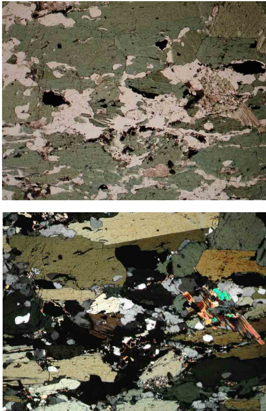
Figure 3.5 Photomicrographs of sample WS995. Amphibole (green mineral) defines the primary fabric. Note the cross-cutting biotite grain on the right. Top: plane polarized light. Bottom: cross polarized light. Width of view is 5mm.
