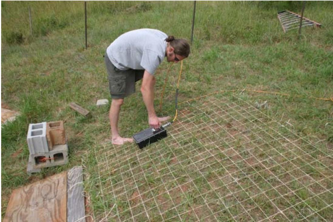
**Figure 20. Antenna operation for GPR survey**
