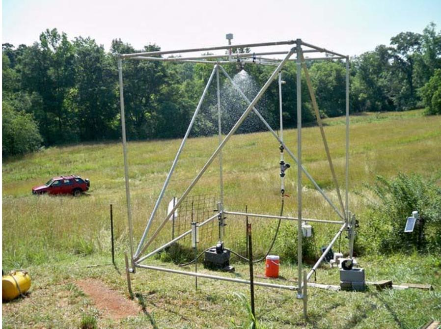
**Figure 19. Tlaloc 3000 sprinkler system over gridded plot**
