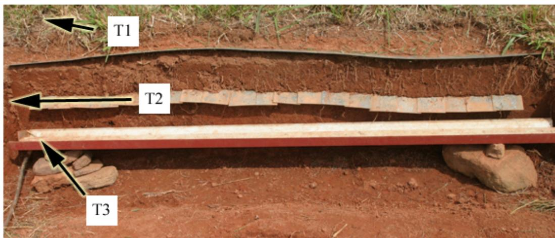
**Figure 16. Location of thermistors relative to the gutter**
