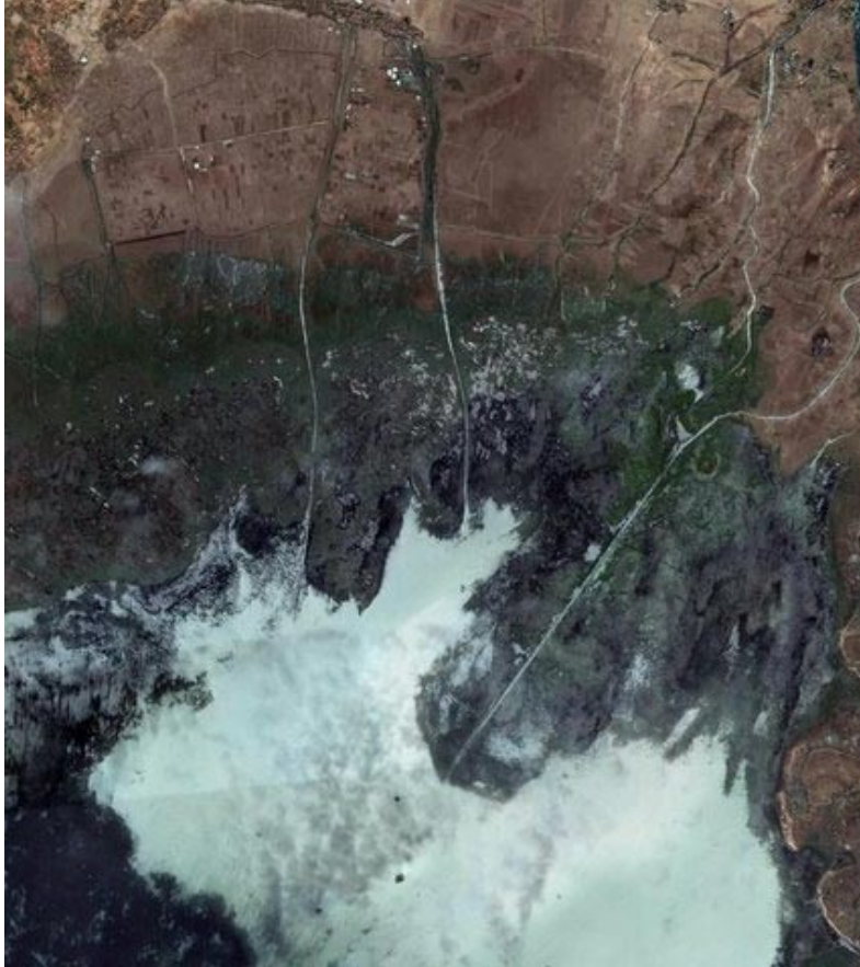
Figure 2.5 Satellite image of the northern sector of Chilika that demonstrates how the lake is shrinking due to siltation. The channel on the right was dredged by the Indian government to maintain access to the Daya and Luna Rivers. The two channels on the left were dredged and are maintained by the local communities that fish in the lake.
