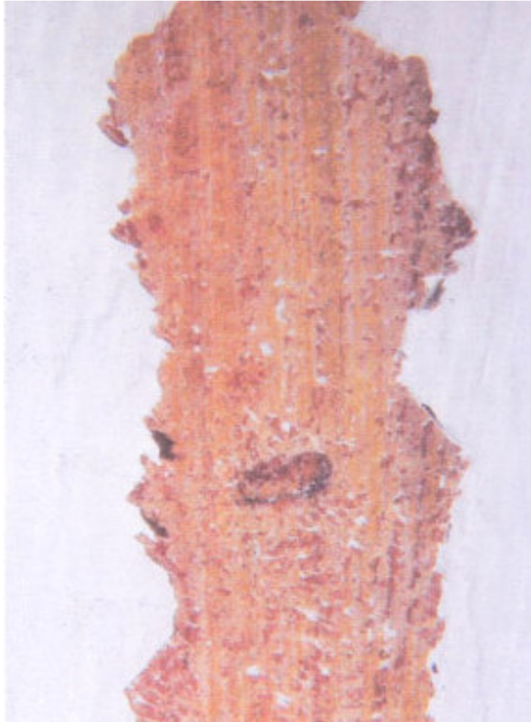
Figure 18: Example of a paint sample showing faux graining. 125
