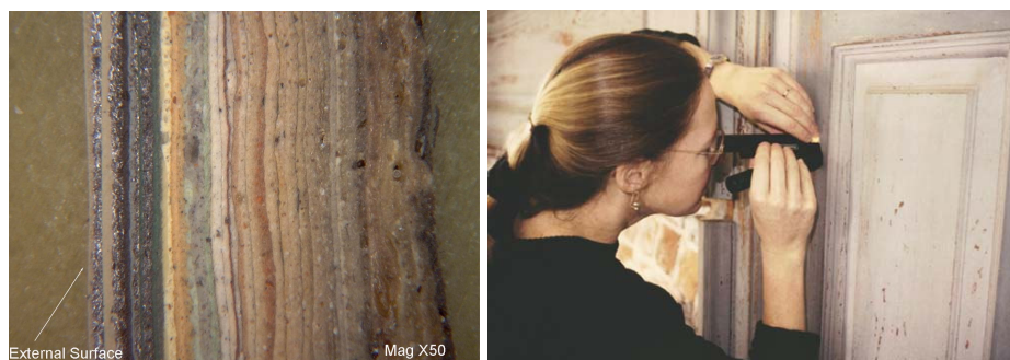
Figure 14 (left): Paint sample at 50x magnification. 116
