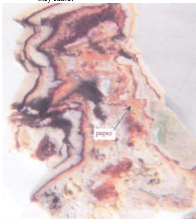
Figure 20: Example of a paint sample showing wallpaper remnants. 127
