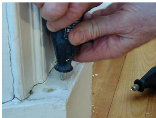
Figure 11: Sampling using a microdrill rather than a knife or scalpel. 109
