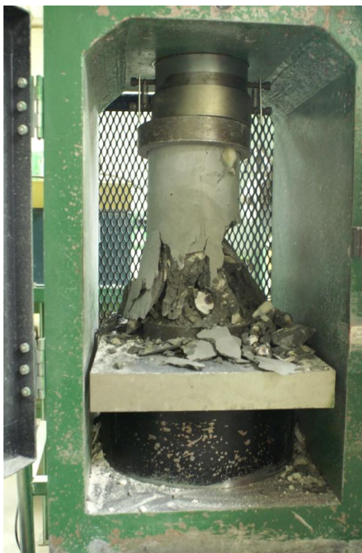
(Figure 23)-Portland mix cylinder
