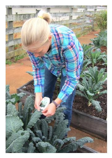
Figure 12. Using the CCM to take a chlorophyll measurement from crop three kale.
