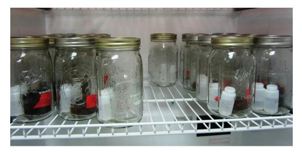
Figure 10. Incubation experiment, respiration of re-wetted substrates.
