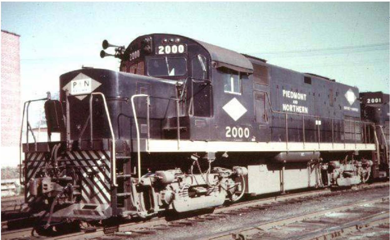
Figure 2.18: The last two locomotives purchased by the P&N were 2000-horsepower ALCO C-420s delivered in December of 1965, Nos. 2000 and 2001. For the first time, the lightning bolt herald disappeared and a new white and chrome yellow diamond logo replaced it. Photo from http://www.rr-fallenflags.org/
