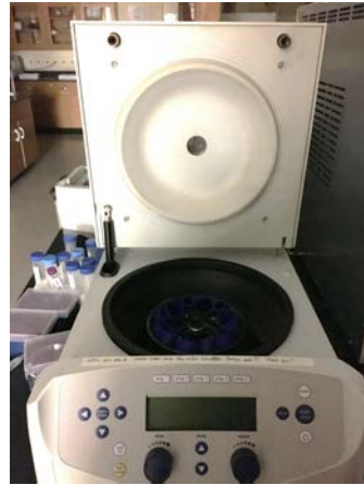
Figure 14 - Centrifuge used to spin cells at low 4°C temperatures.
