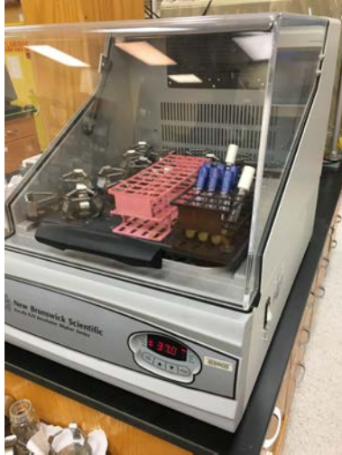
Figure 12 - 37°C, 290rpm Shaker Incubator.
