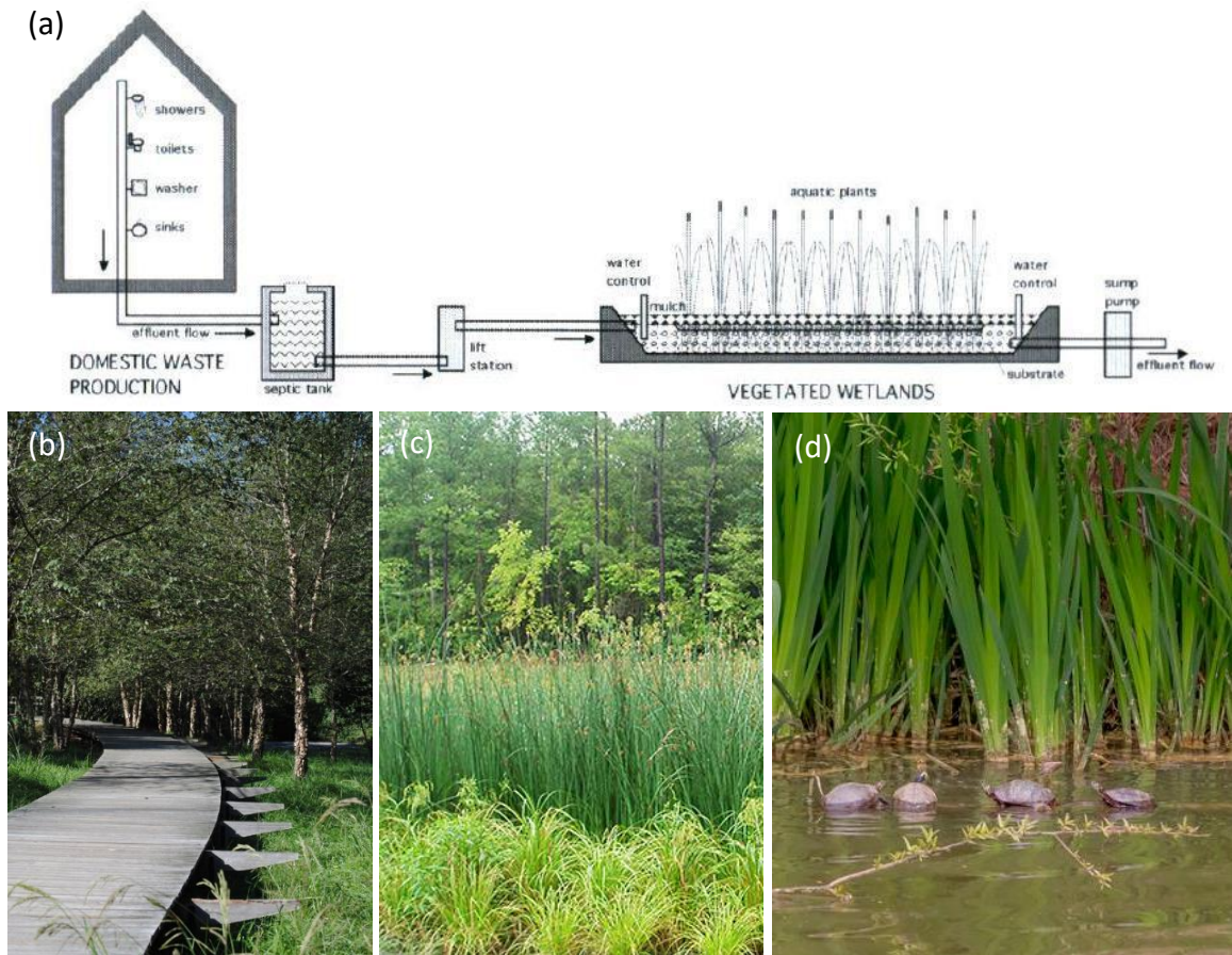
Figure 4.12 Constructed Wetlands: a) Conceptual section diagram; b) Boardwalk; c) Vegetated wetlands; d) Turtles in wetlands (Source: Diagram drawn by Phillip Tabb; Photograph by Yingting Chen)
