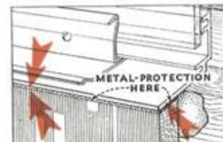
7. PROTECTION FOR CARRARA A sturdy, square-cut, continuous metal flange projects over edge of Carrara, shielding the area which is most vulnerable.
