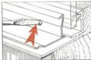
4. INSTALLATION OPERATIONS ALL FROM OUTSIDE Both glass and sash are set from outside by standard wood or machine screws. No special keys or tools required.
