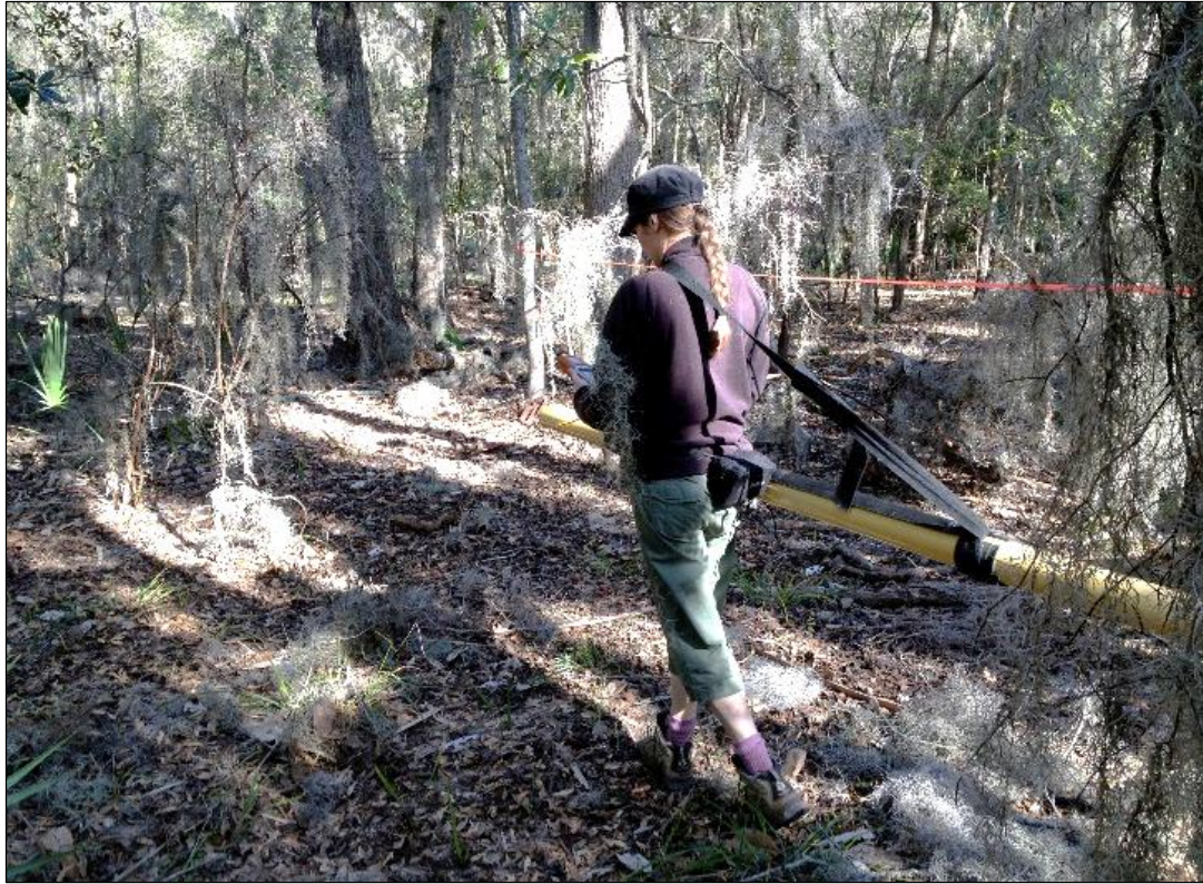
Figure 3.7: Author surveying a forest site with the Dualem 2S™ EMI. As shown, EMI was carried at hip height.
