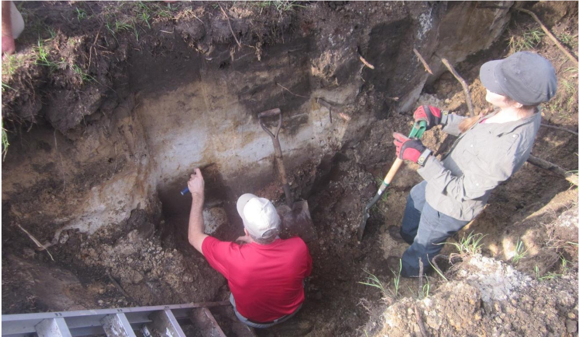
Figure 5.5: Assessing the best way to extract the soil profile chosen for making the monolith.
