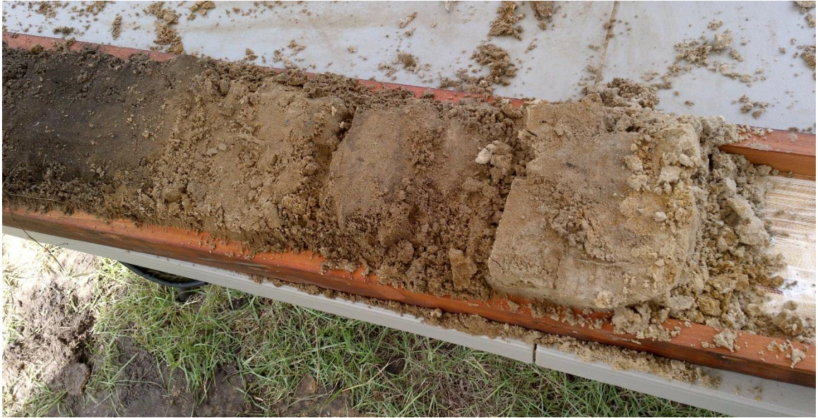
Figure 5.7: Placing the fragile pieces of the soil profile into the frame.
