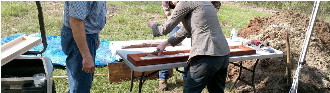
Figure 5.3: Adding a layer of cheese cloth and glue to the bottom of the frame, before adding soil.
