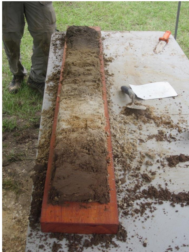
Figure 5.8: The entire profile is pieced within the frame and ready for final preparation.
