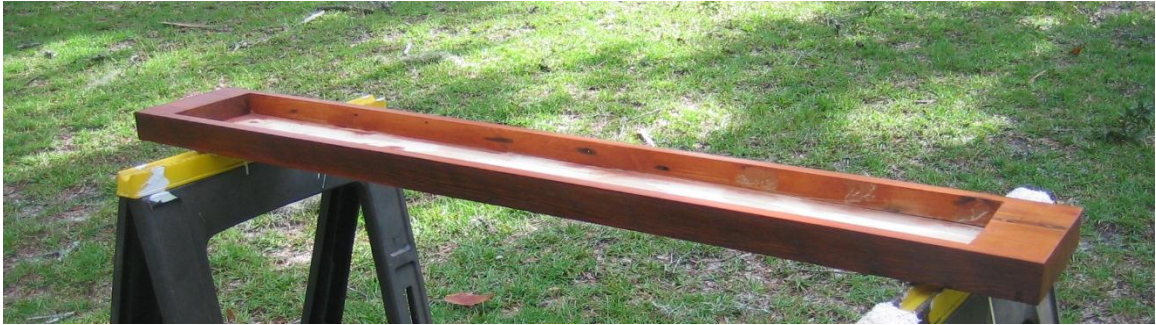
Figure 5.2: Soil monolith frame.
