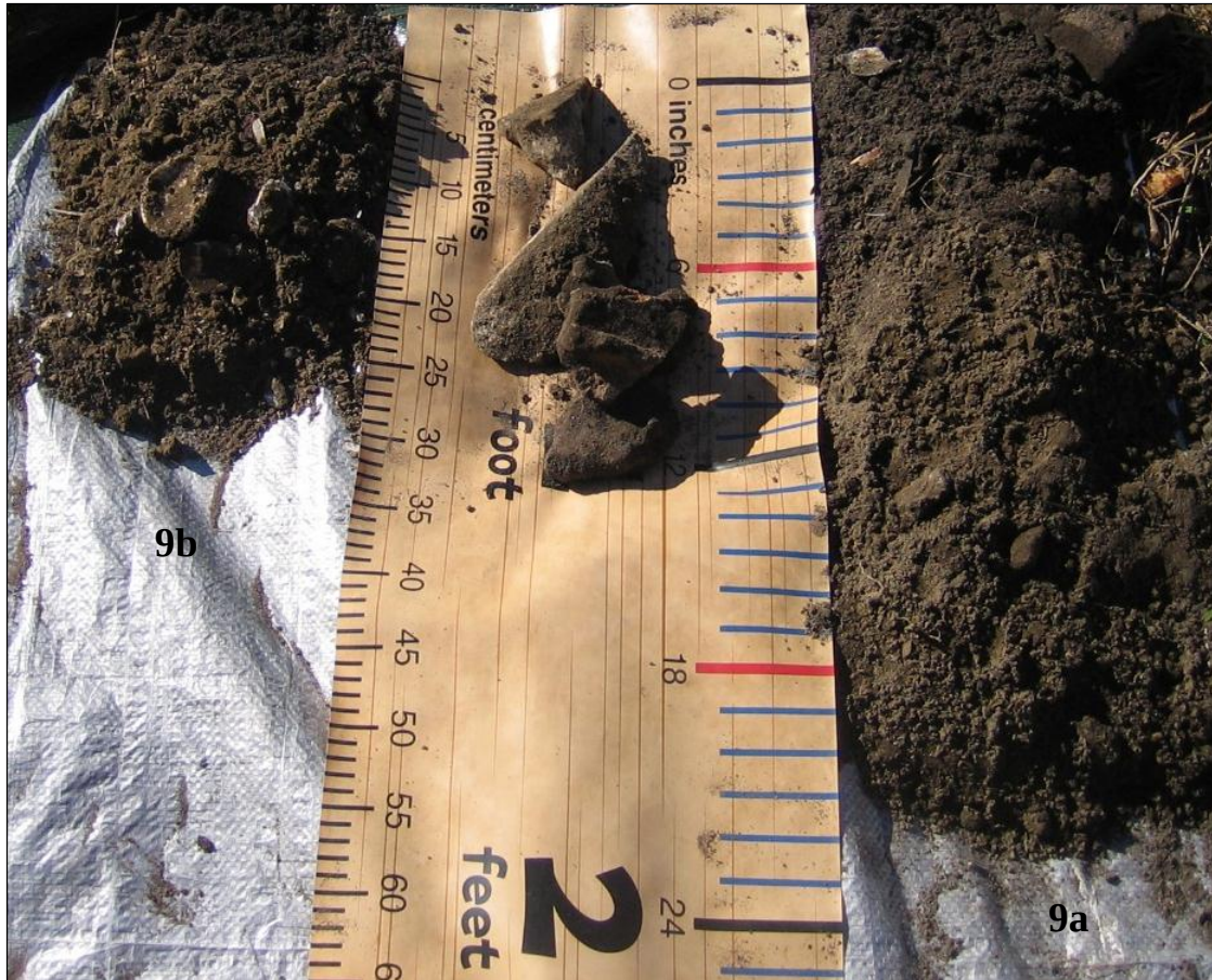
Figure 3.21: Image displays soil profiles of samples 9a and 9b. Debris (concrete, brick, gravel, shells, charcoal) prevented further soil excavation beyond a 25 cm (9b) and 50 cm (9a) depth.
