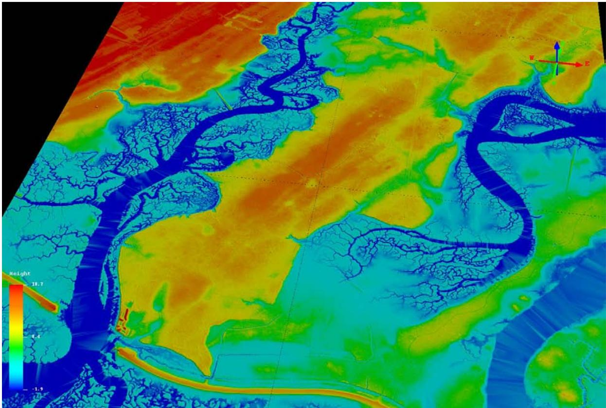
*Figure 3.2. Lidar derived DEM of Wormsloe. Relief varies little across the study site with the minimum elevation being 1.5 m (shown in green) and the maximum elevation being 4.5 m (shown in red).*
