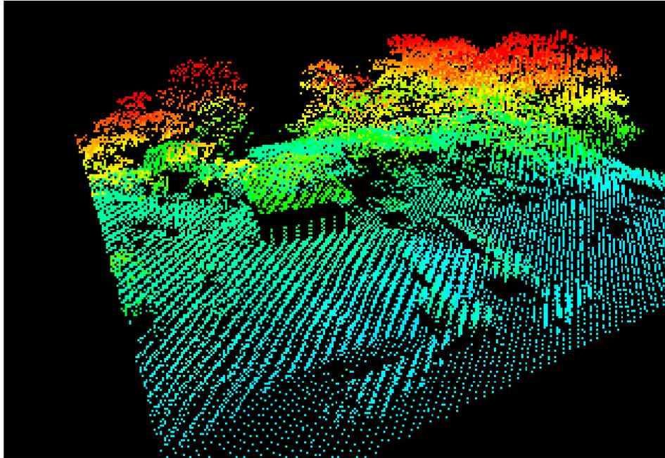
*Figure 2.4. Perspective view of lidar point cloud data showing rooftops and trees for an area on the Isle of Hope, Georgia.*
