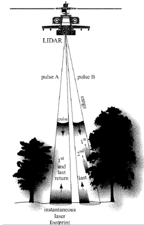
Figure 2.5. Multiple returns may be generated from a single lidar pulse (From Jensen, 2006).
