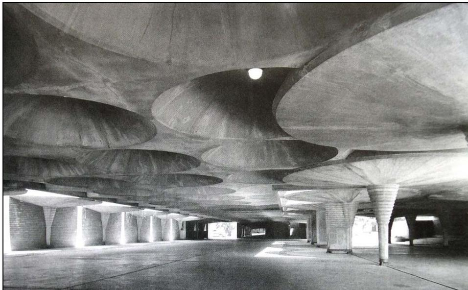
Figure 23: The Carport in the SC Johnson Building (Note the shorter dendriform column)
