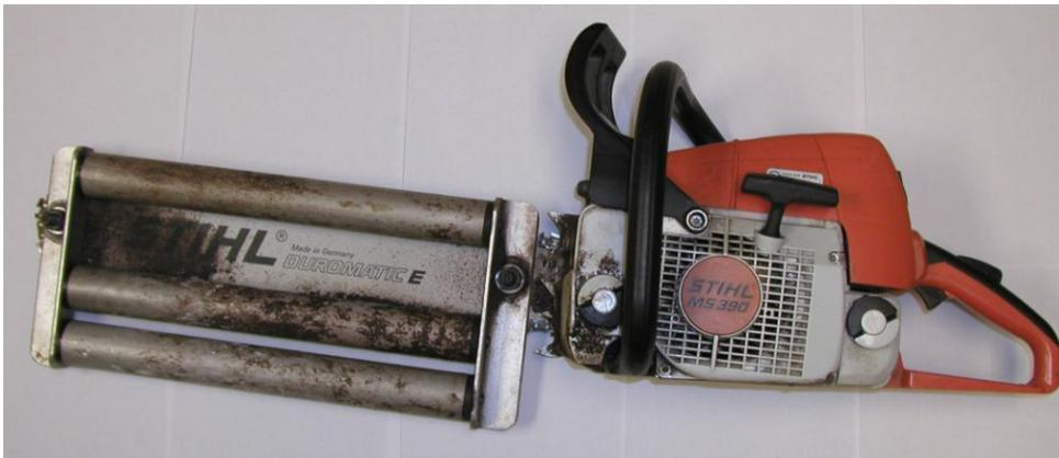
**Figure 2.1** – Chainsaw with specialized attachment. Used to cut discs of an exact thickness.
