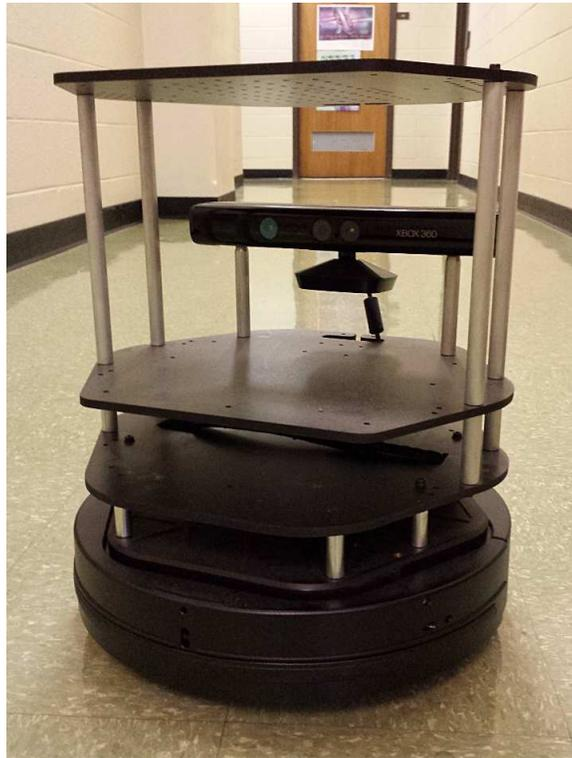
Figure 1.1: A Turtlebot 2, used in our robotic experiments. As an example of an inexpensive autonomous differential drive robot it exhibits noisy, limited sensors and imperfect actuators.
