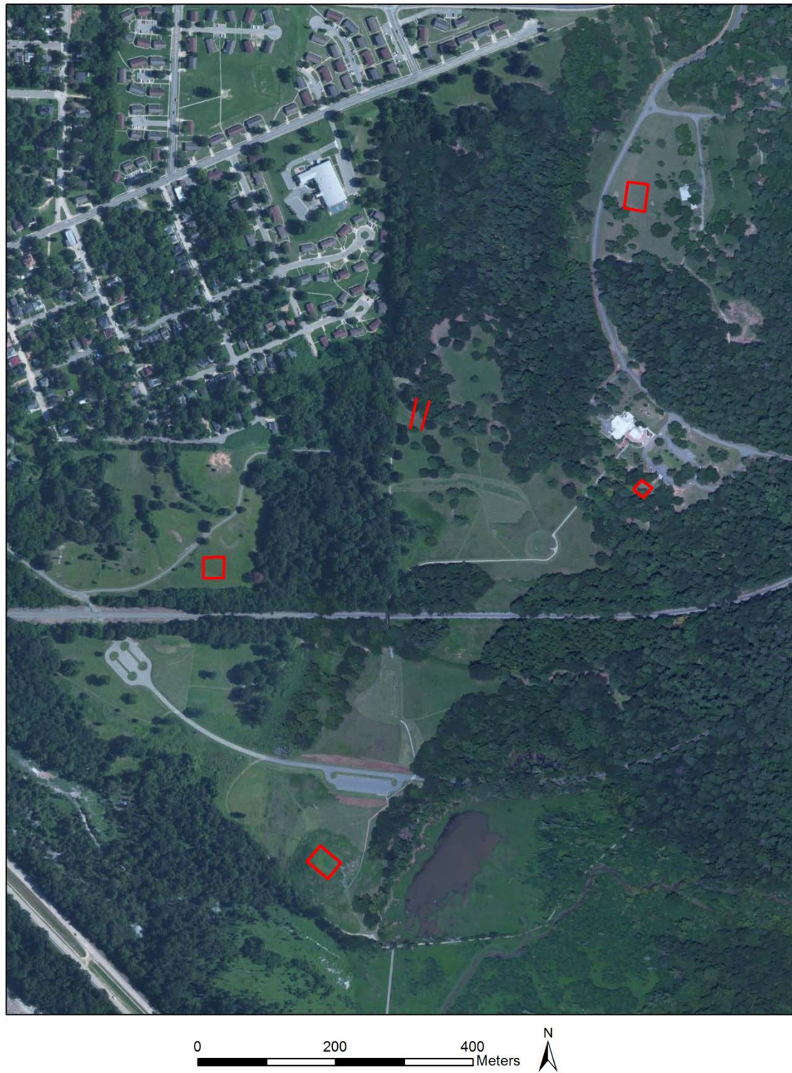
Figure 2.5. Locations of blocks and transects I collected with a SIR-2000 GPR and 500 mHz antennae (2010 Bing Maps image).
