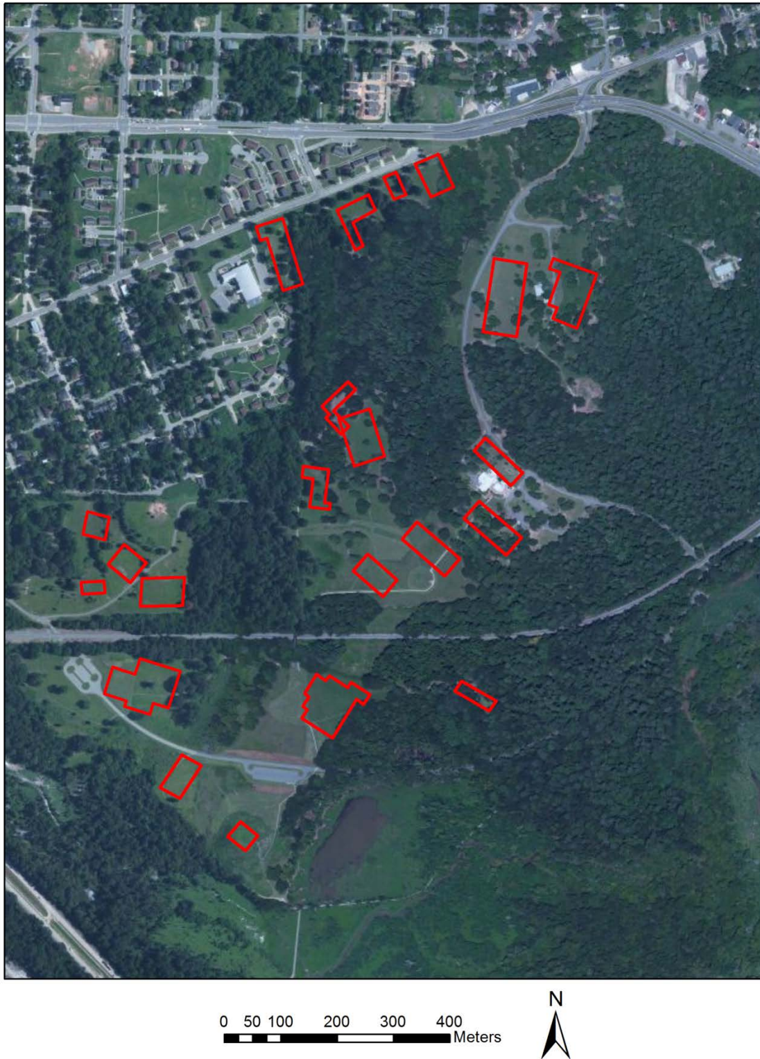
Figure 2.4. Locations of survey blocks I collected with a GEM-300 conductivity meter at 12150 Hz (2010 Bing Maps image).
