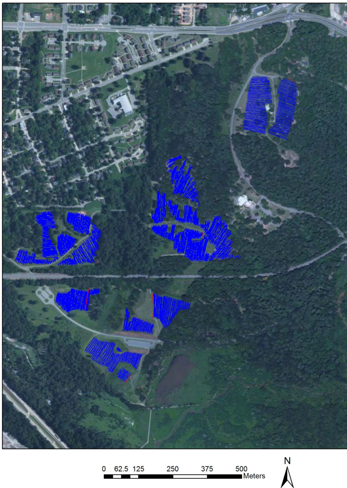
Figure 2.3. Locations of traces I collected with a GPS guided cesium vapor magnetometer (2010 Bing Maps image).
