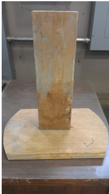
Figure 5.5 – Picture of Compaction Tool used on demo units
