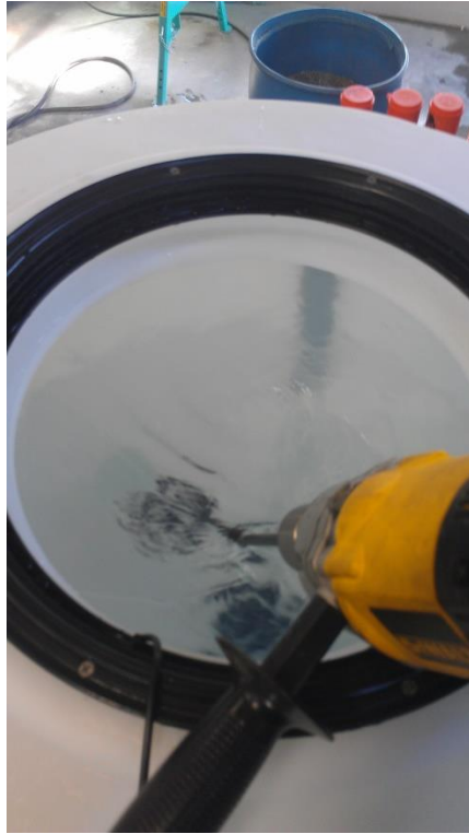
Figure 5.6 – Mixing Synthetic Stormwater using drill and paddle
