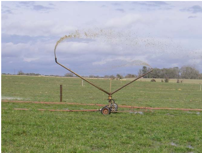
Figure 5.2: The land application system, or 'slurry slinger', connected to the storage tank.
