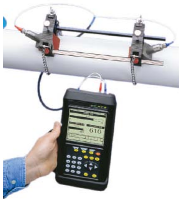
Figure 4.2: The non-invasive flowmeter used for this project.
