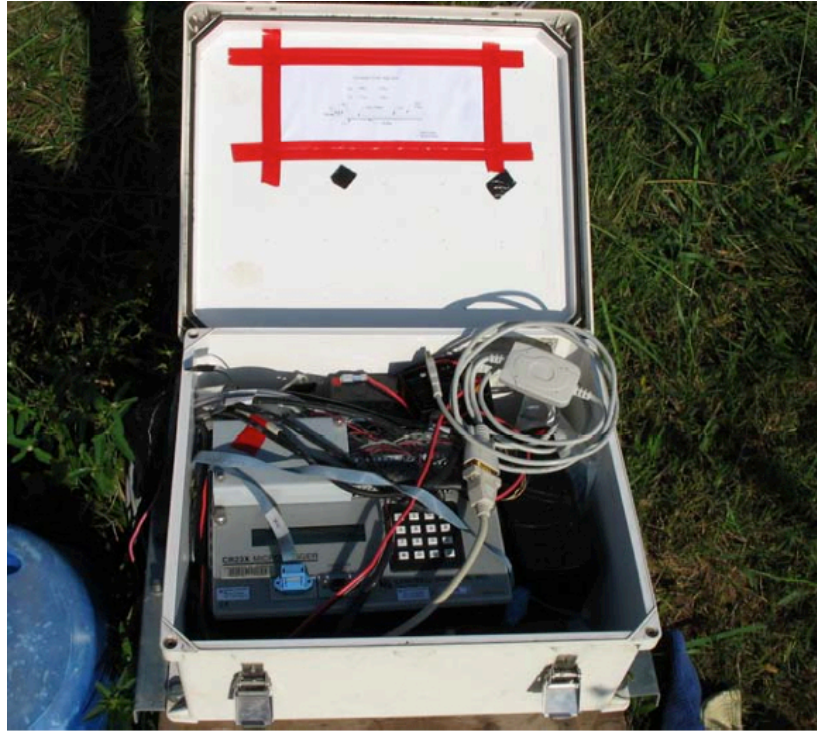
Figure 11: Campbell Scientific CR23X datalogger wired to thermistors.
