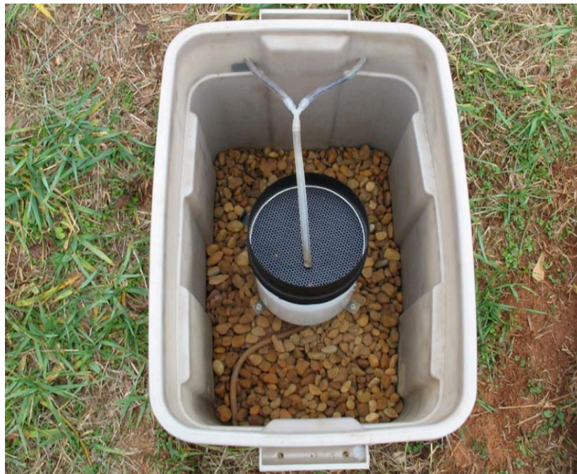
Figure 10: ONSET tipping bucket rain gauge located downhill of trench.
