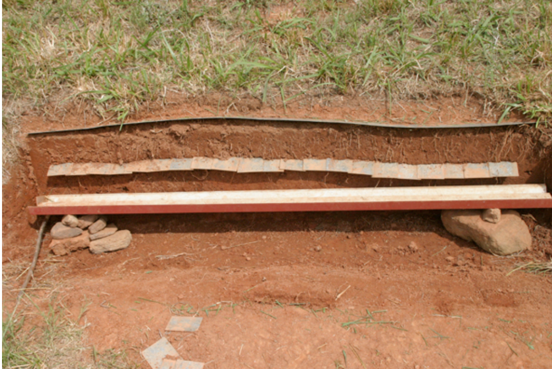
Figure 8: Gutter setup. Note metal flashing to prevent overland flow into gutter and steel drip plates pounded into cut soil face at approximately 10 cm to promote flow into the gutter.
