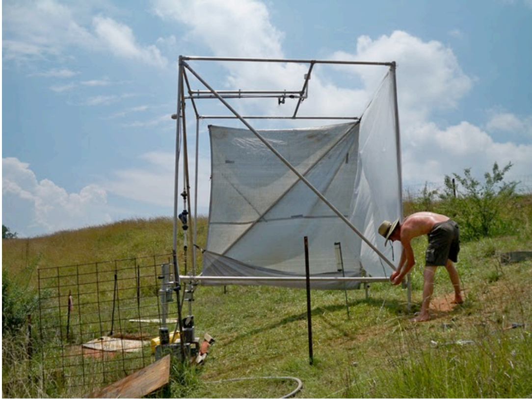
Figure 7: Rainfall Simulator set up over study plot. Note rain gauge to quantify rainfall rate.
