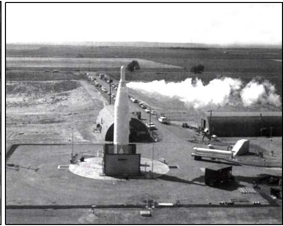
Fig. 5-3: An Atlas F ICBM being raised from its silo in a fueling exercise (Gibson 1996, p. 13)
