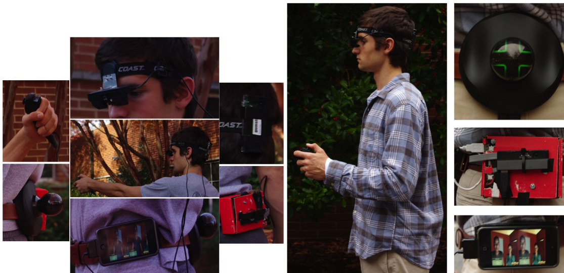
Figure 3.3: (Left) A user within the low-cost, portable, immersive virtual environment outdoors. (Right) Components hidden under the shirt of the user on a belt: an electromagnetic tracking source, single board computer, and smart phone.
