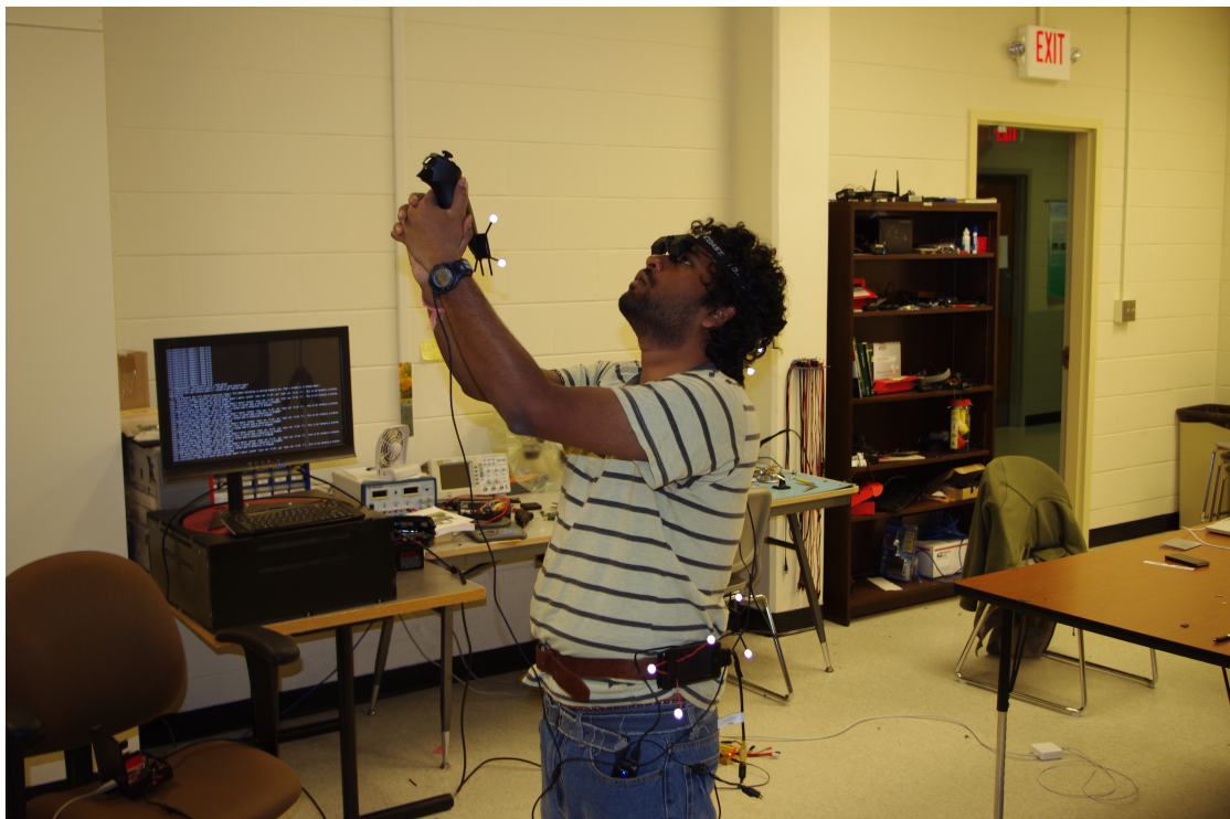
Figure 2.2: This is an example of a real-time position tracking using a five camera OptiTrack system (Flex 3 cameras) with retro-reflective markers being tracked at 100 FPS. This picture is courtesy of the Virtual Experiences Lab at UGA.
