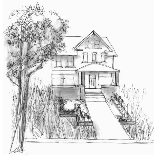
Figure 5.6: Possible house entrance 2. Narrow raised vegetable garden plots, easily accessible from front walk, are made of materials compatible with the house and the pillars of the porch.
