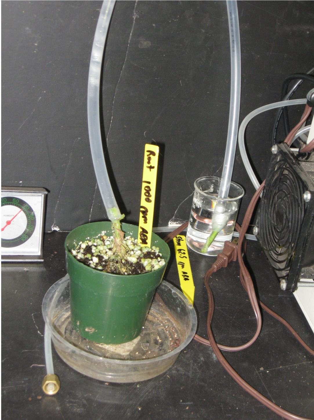
Figure 4.2. An image of how root systems and stem sections were sealed to the tubing for conductance measurements.
