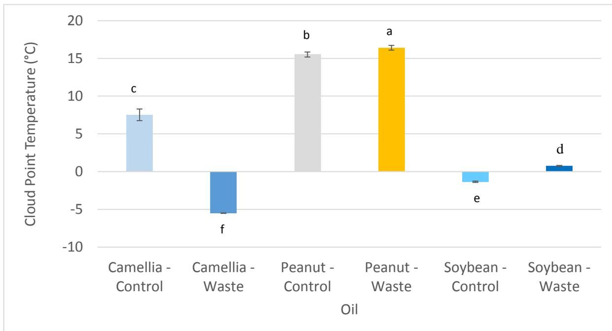
**Figure 4.2: Cloud point temperature of control and waste biodiesel products for Camellia, peanut, and soybean oils ( $p \leq 0.001$ )**
