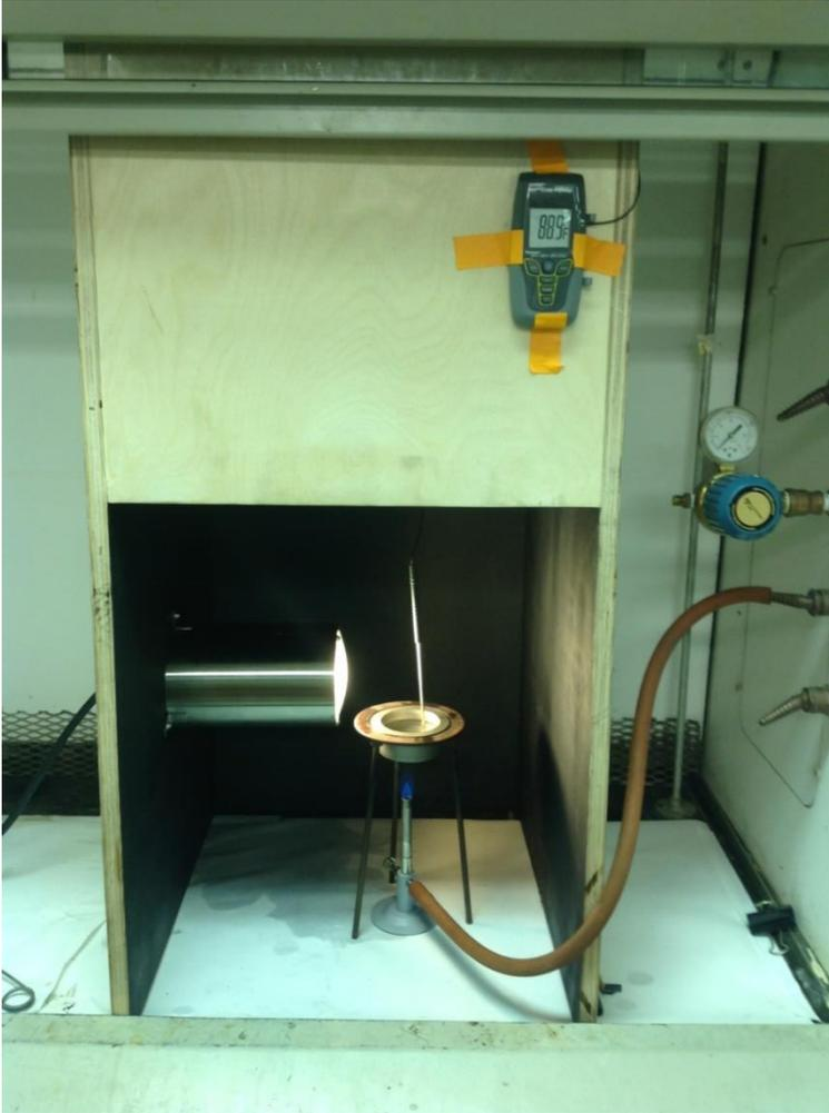
**Figure 2.1: Smoke point testing apparatus**
