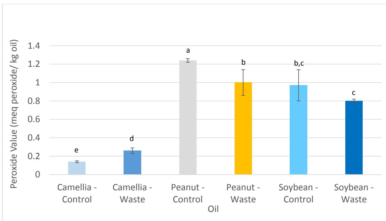
**Figure 4.3: Peroxide values (PV) of control and waste biodiesel products for Camellia, peanut, and soybean oils ( $p \leq 0.001$ )**
