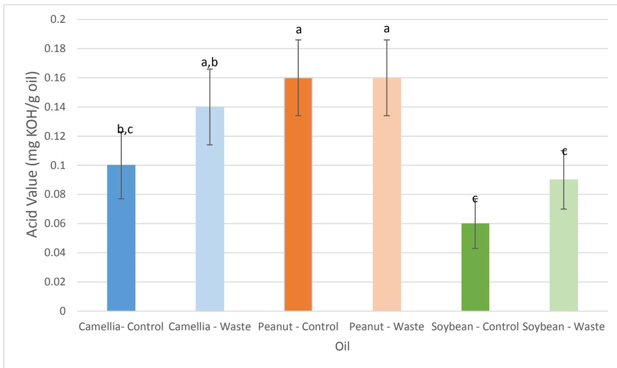
**Figure 4.4: Acid values of control and waste biodiesel products for Camellia, peanut, and soybean oils ( $p \leq 0.001$ )**
