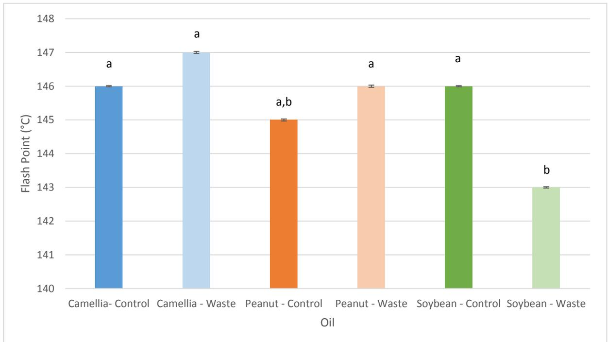
**Figure 4.1: Flash point temperature of control and waste biodiesel for Camellia, peanut and soybean oils ( $p \leq 0.002$ )**
