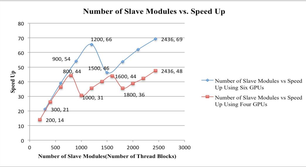
Figure 3.6: The relationship between number of thread blocks (slave modules) to be solved on the device and the speed up. The drop in the speed up is due to exceeding the maximum number of TBs running simultaneously on the device, given that the time of the CPU is monotonically increasing.
