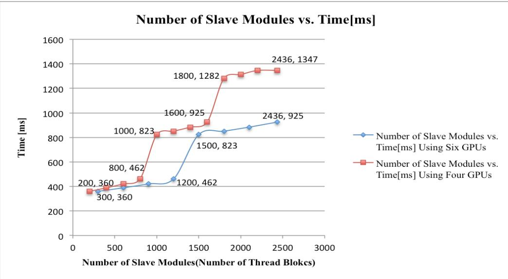
Figure 3.5: The relationship between number of thread blocks (slave modules) to be solved on the device and the required time. The jump in time is due to exceeding the maximum number of TBs running simultaneously on the device. If GPU is capable of running several N blocks simultaneously. Then from 1 to N blocks takes same time to complete.
