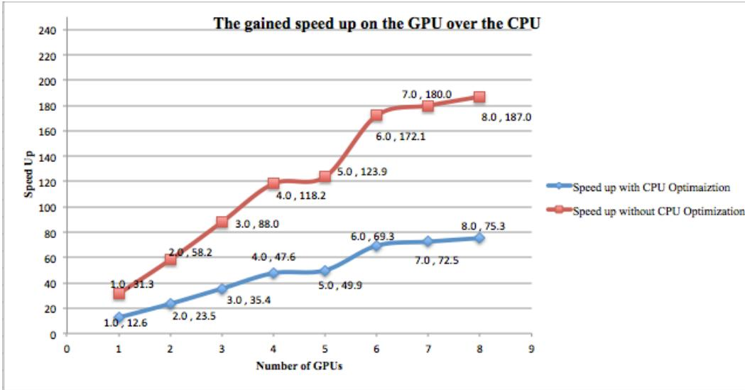
Figure 3.4: The achieved speed up using Multi-GPU [NVIDIA Kepler K-20x Tesla] over an extreme edition of CPU [Quad-cores CPU [Intel(R) Core(TM) i5-2400 CPU@ 3.10GHz]. Red line shows the speed up without using the `-O2` and `-O3` flags for CPU optimization(C++ code/g++ compiler) and blue line shows the speed up with using `-O2` and `-O3` flags for CPU optimization.
