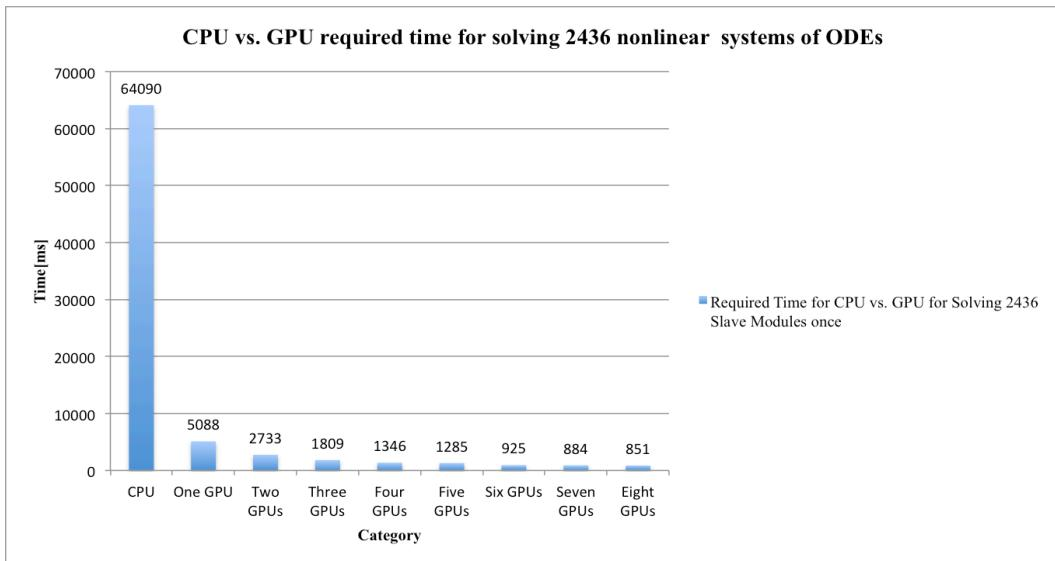
Figure 3.3: The time required for solving 2436 slave modules just one time using a NVIDIA GPU(s) [Kepler K-20x Tesla] over an extreme edition of optimized CPU [Quad-cores CPU [Intel(R) Core(TM) i5-2400 CPU@ 3.10GHz]. Using four of the GPUs to solve our target genetic network 800,000 times shown in the Figure (3.2) to fit the observed data requires just twelve days while using the CPU requires a year and six months.
