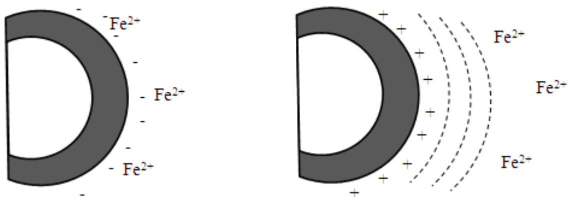
Fig. 5. When the surface charge of an oil droplet and prooxidant are opposite, oxidation is promoted. However when the surface charge of an oil droplet and prooxidant are the same, repulsive forces are generated that retard oxidation.
