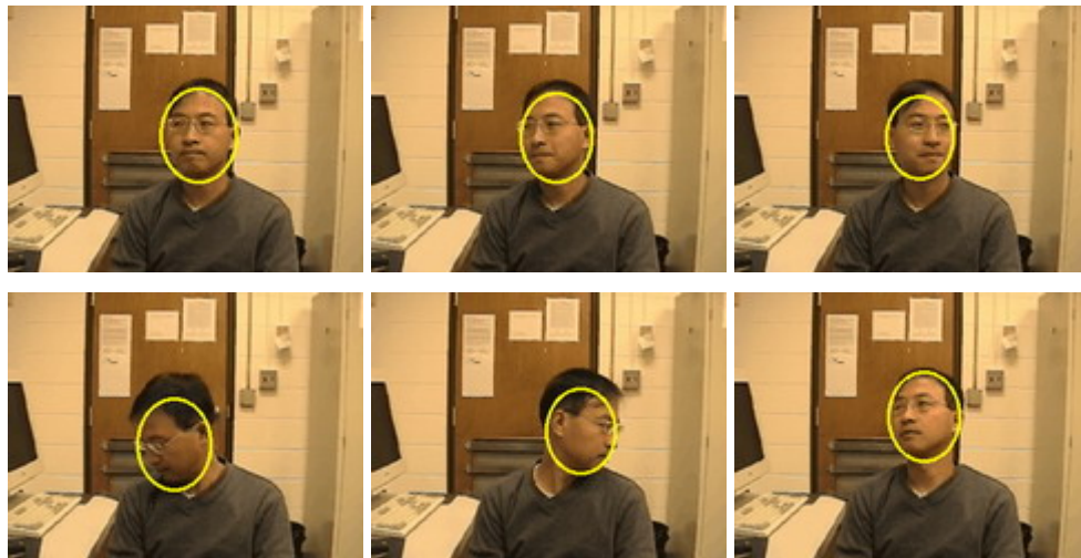
Figure 3.14 Tracking results with the BAPF at six different times in test video 3. From top left to bottom right, the frame numbers are 12, 40, 61, 136, 158, and 180.
