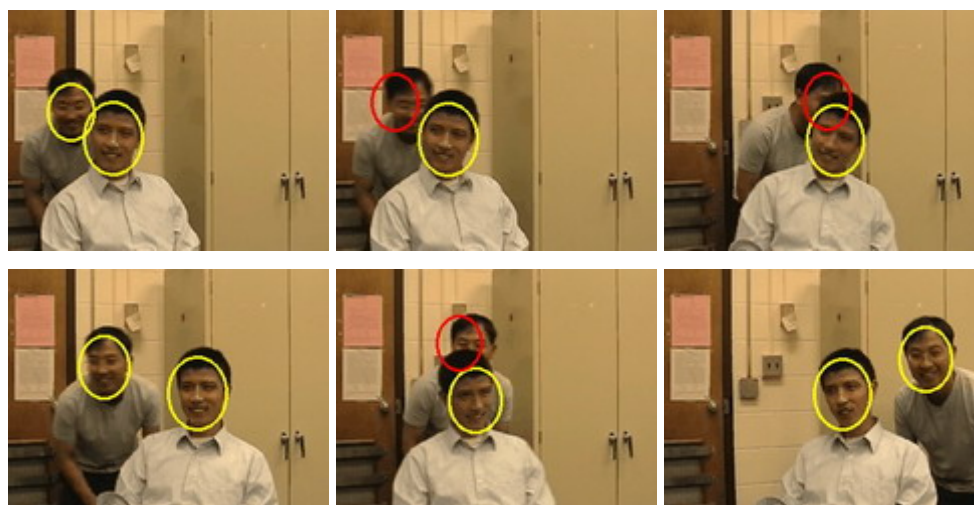
Figure 3.13 Tracking results of two faces in test video 2. Yellow ellipse means that no occlusion has occurred, while red ellipse means occlusion has occurred. From top left to bottom right, the frame numbers are 2, 4, 25, 38, 78, and 138.
