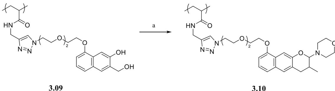
Reagents and Conditions: a) isobutyraldehyde, morpholine, *p*-toluenesulfonic acid, 310nm hv, acetonitrile/water 1:1.
