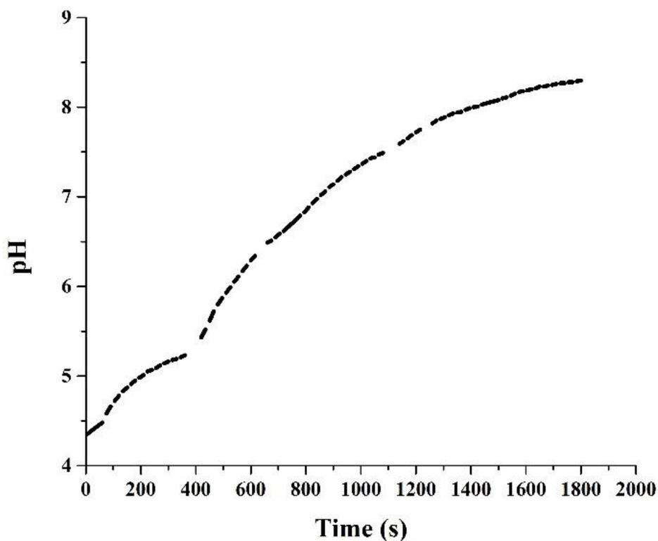
**Figure 2.03.** Hydrochloric Acid Neutralization by Propylamine Released from NQMP-Photobase under Pulsed Irradiation.
