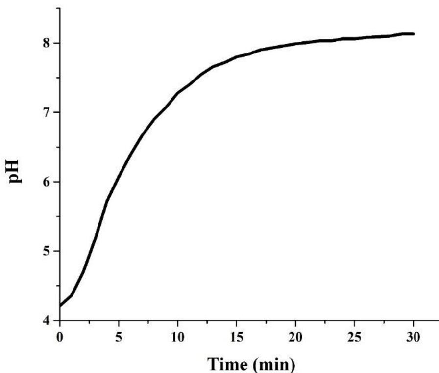
**Figure 2.02.** Hydrochloric Acid Neutralization by Propylamine Released from NQMP-Photobase under Constant Irradiation.
