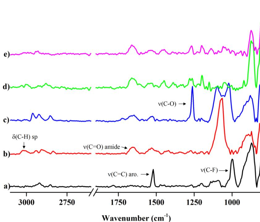
**Figure 3.04.** FTIR Spectra of Silicon Substrates with a) Poly(PFPA), b) Poly(Propargyl Acrylamide), c) Surface-Tethered Protected NQMP, d) Surface-Tethered NQMP, e) Surface-Tethered NQMP after Isobutyraldehyde Conjugation.
