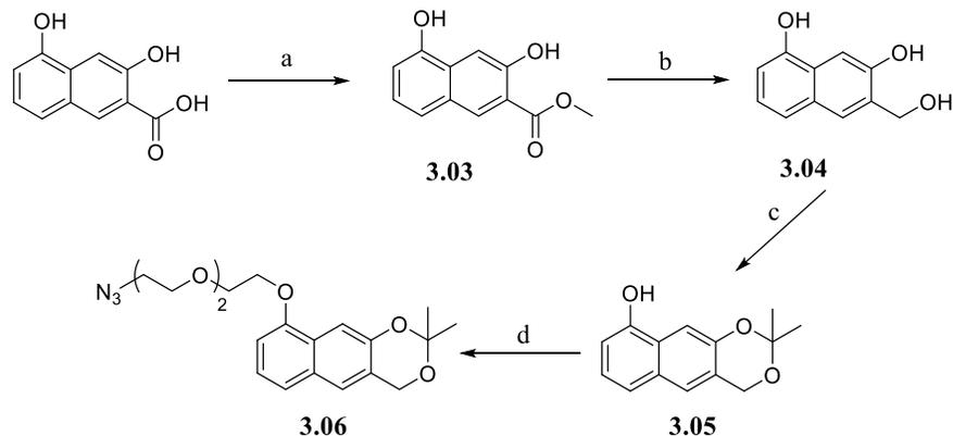
Reagents and Conditions: a) H<sub>2</sub>SO<sub>4</sub>, methanol, 97%; b) DIBAL, THF, 91%; c) 2,2-dimethoxypropane, p-toluenesulfonic acid, acetone, 95%; d) **3.02**, K<sub>2</sub>CO<sub>3</sub>, DMF, 55%.
