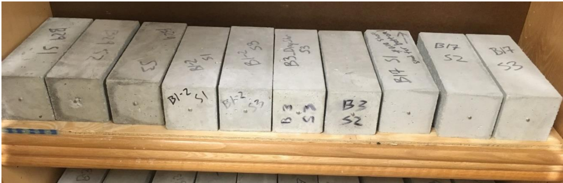
Figure 18: Drying shrinkage prisms
