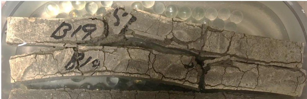
Figure 37: Deleterious expansion by sulfate attack of MK2-10 mortar bars
