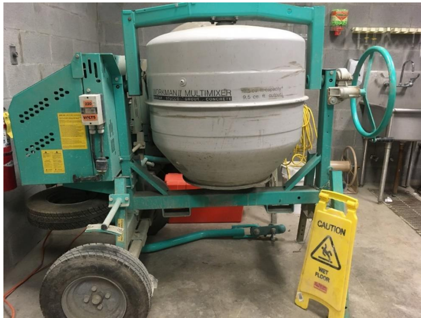
Figure 11: Mixer used in concrete batching
