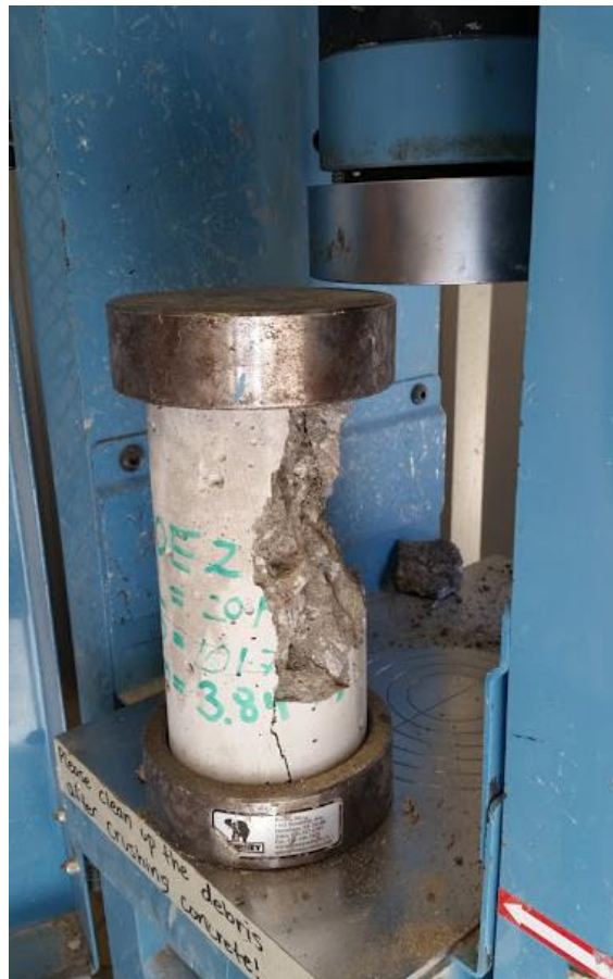
Figure 14: Fractured compressive specimen
