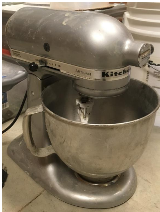
Figure 12: Mixer used in mortar batching
