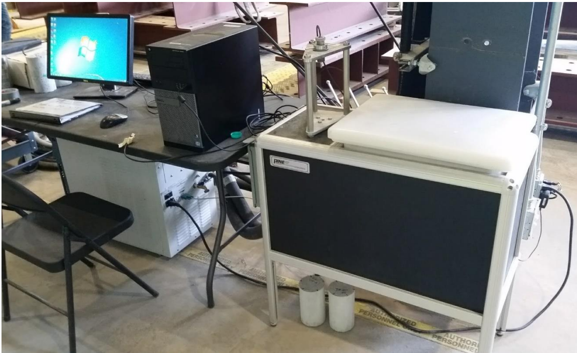
Figure 20: CTE testing machine
