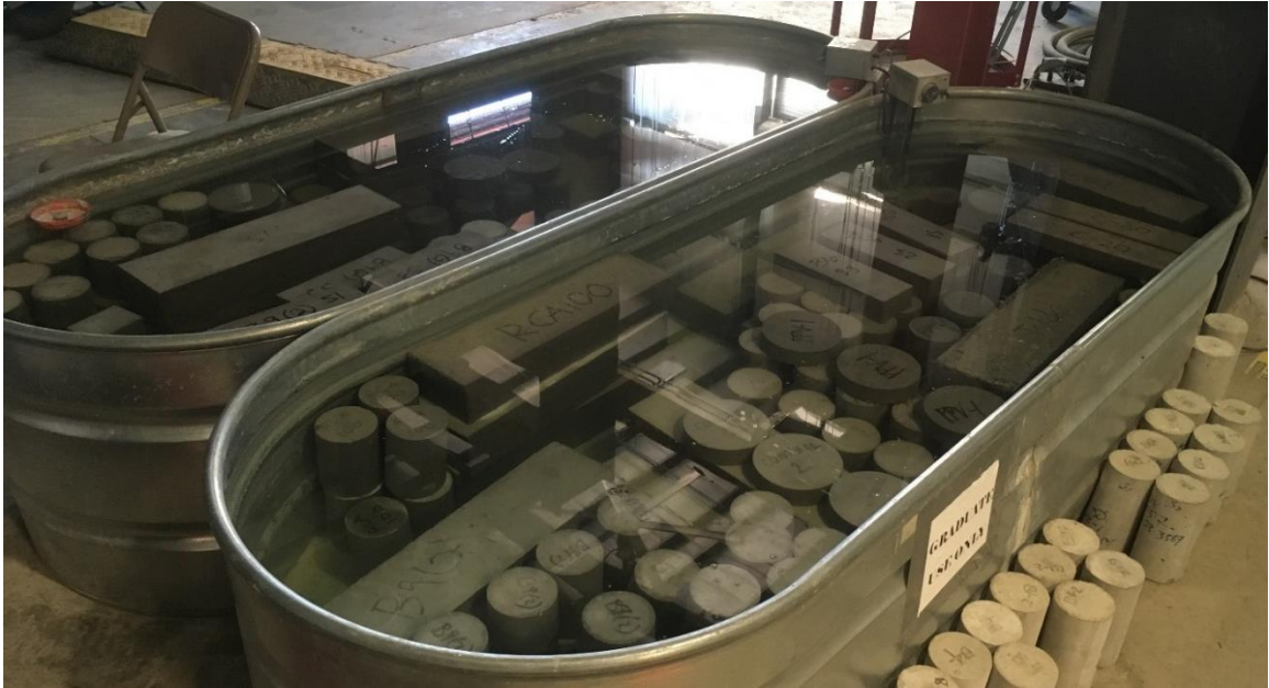
Figure 13: Lime-saturated curing tank
