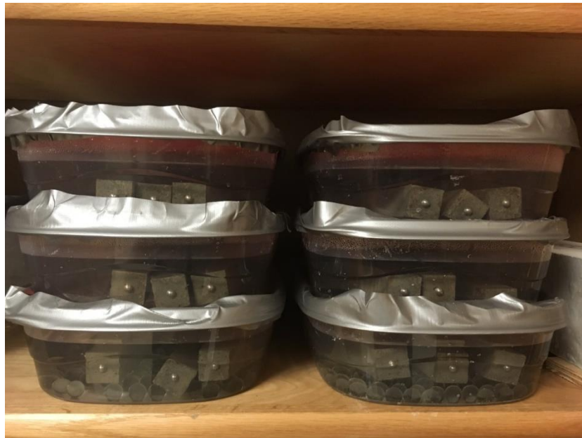
Figure 17: Mortar bars in sulfate solution
