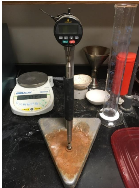
Figure 19: Length comparator used in sulfate, ASR, and shrinkage tests
