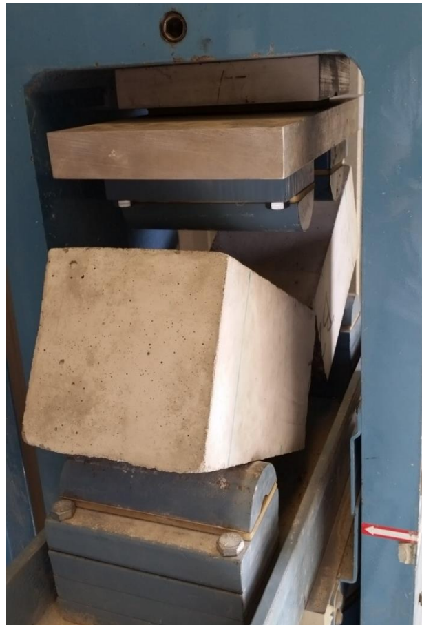
Figure 15: Fractured MOR specimen
