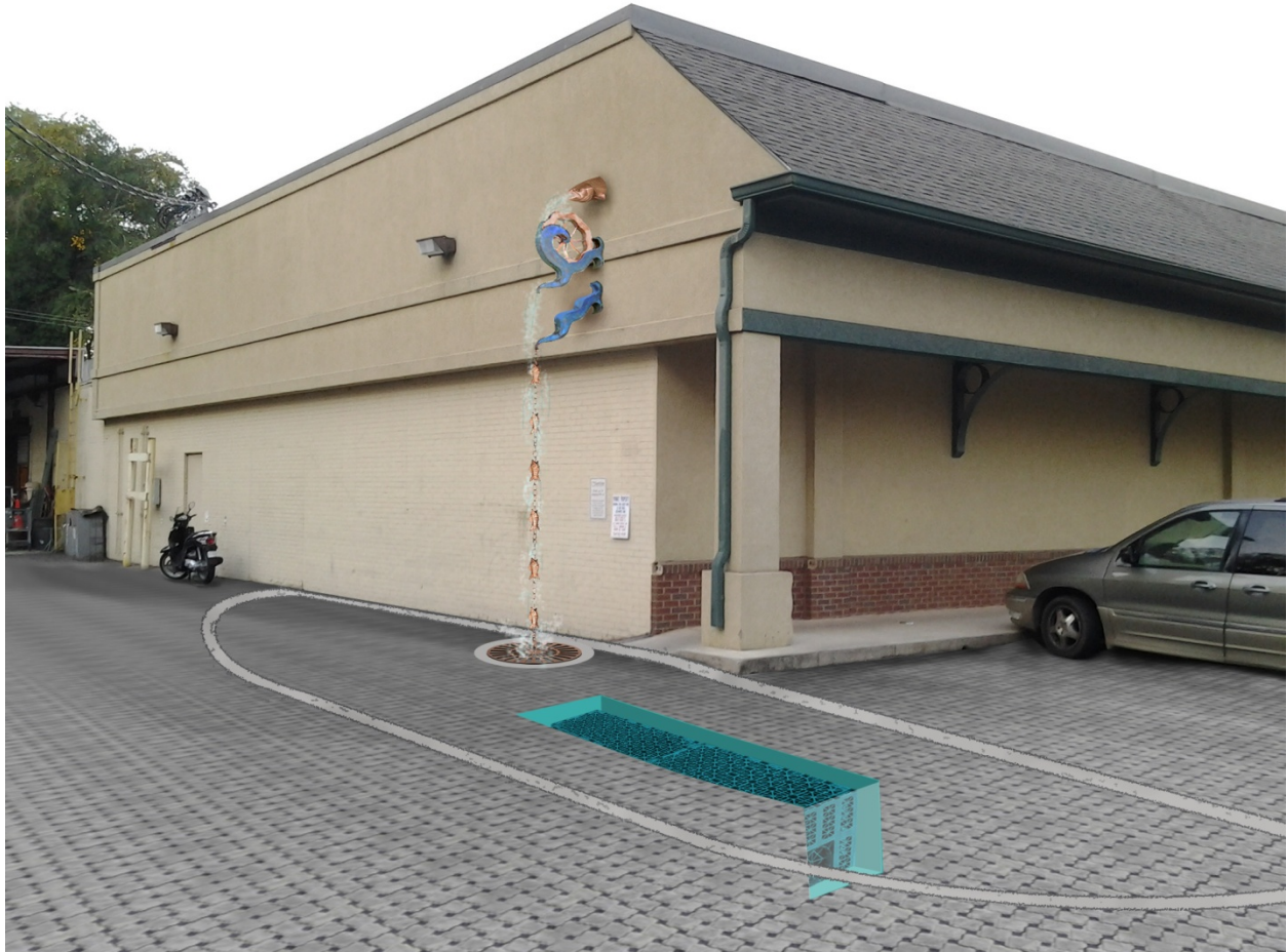
Figure 5.23 - Fanciful rain chain with kinetic water sculpture as part of cistern delay system
