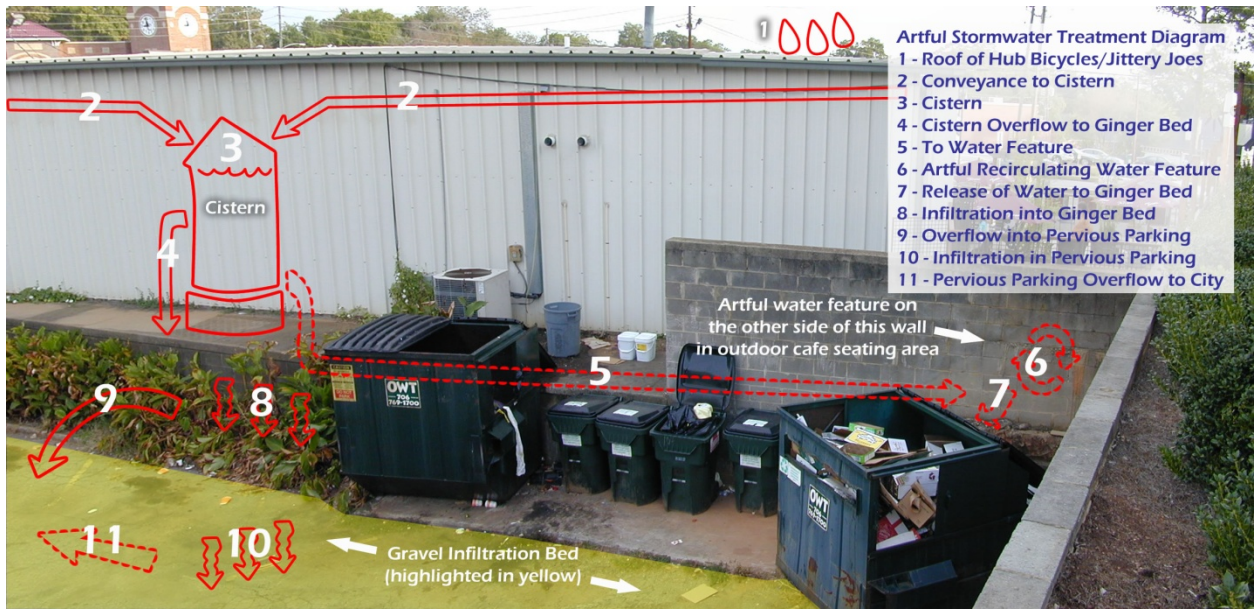
Figure 5.10 - Artful stormwater treatment diagram for Jitter Joe's water feature
