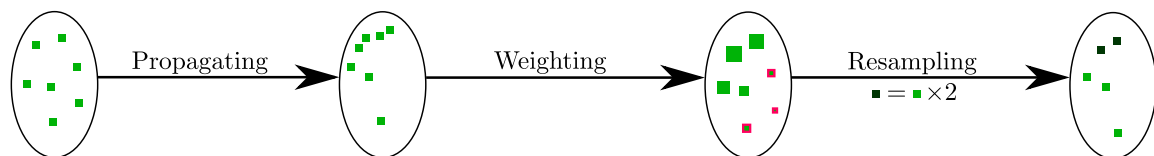
Figure 3.2: Propagation, weighting and resampling steps in particle filtering method on a sample set. The initial particles will be updated based on the action of the robot. After the propagation step, the sensory data helps in weighting each one of the particle in the sample set. Finally, a resampling according to the weights of each particle will generate the sample set used in the next iteration.
