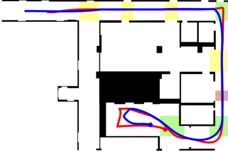
Figure 5.3: Robots' paths in the third experiment taken by the leading robot (red), the follower robot (blue) and the third robot (green). The robots start from the top-left corner of the map and continue on the paths indicated on the map to get to the blocked area. After facing the wall at the blocked area, both robots will take a U-turn and follow the same path back to the start point. Depicted paths are actual paths the robots have taken in one of the simulation experiments we performed. The colored areas in the map show different features of the map such as turning point (green), cross-walks (red) and intersections (yellow).
