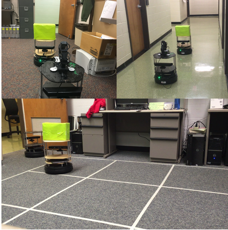
Figure 5.9: Turtlebot II robots from the start point (top-left picture) to their destination (bottom picture) which is the grid shown in the figure.
