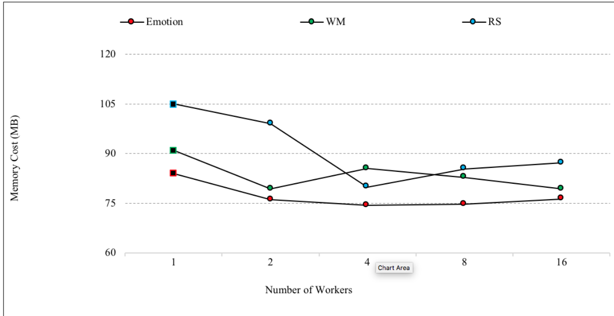
Figure 3.10. Memory cost for decomposing three different fMRI datasets by recruiting varying number of workers, using the AWS-EC2 solution. The results from single-worker (standalone mode) configuration are highlighted as blocked markers.
