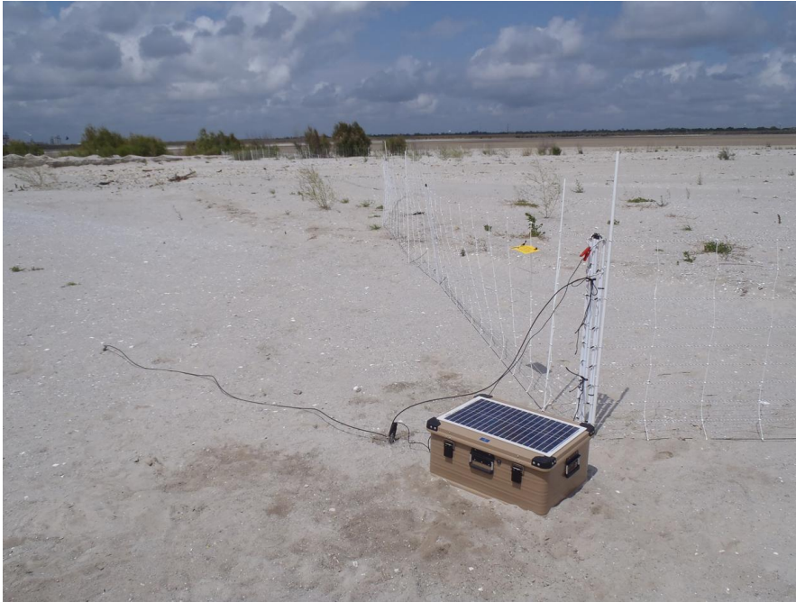
Figure 4.1. Premier Pos-Neg® electric mesh fencing with solar-powered energizer, installed along the perimeter of a least tern colony in Georgia in 2012. Electric fencing of this kind greatly increased nest success at least tern colonies in Georgia by minimizing nest predation by mammalian predators.
