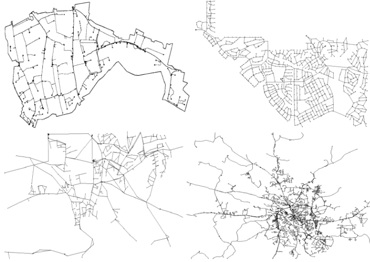
Figure 2.2. Real-world water distribution networks reported by Yazdani and Jeffery [9]: East-Mersea (top-left), Colorado Springs (top-right), Richmond (bottom-left) and Kumasi (bottom-right).
