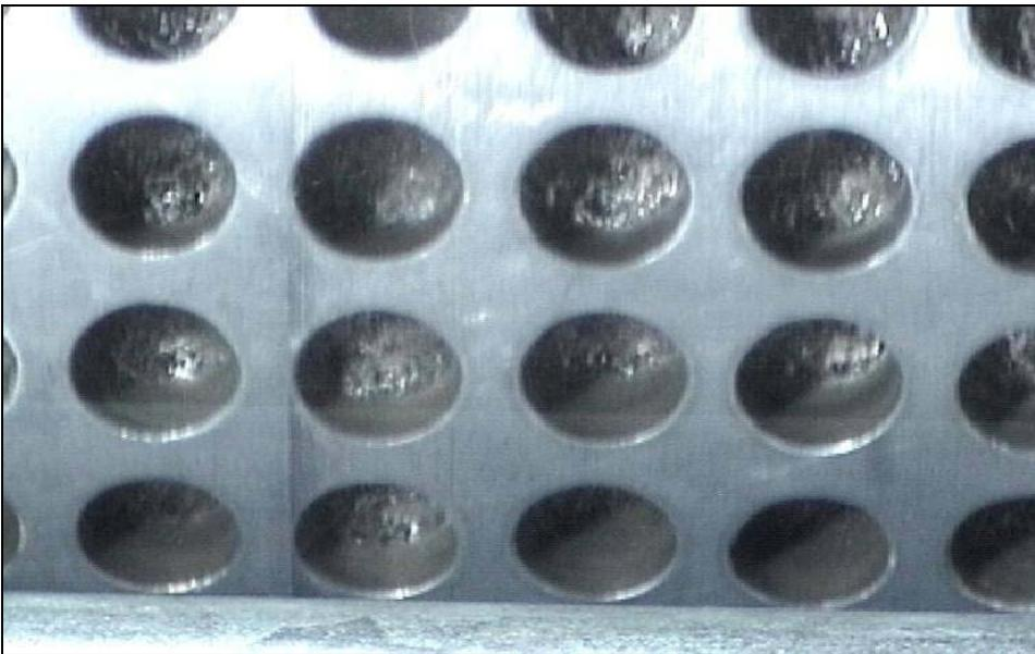
Fig.2.3 - Hydrodynamic cavitation within inner rotor cavities (Reproduced with permission from Hydrodynamics Inc. Rome, GA).
