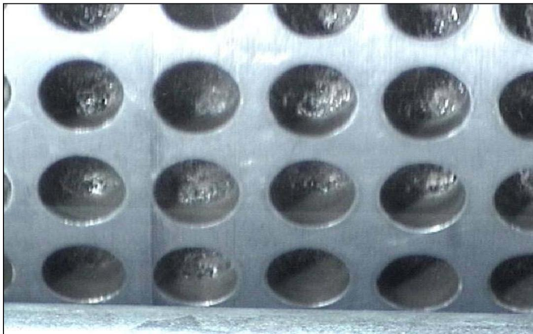
Fig.3.3 - Hydrodynamic cavitation within inner rotor cavities (Reproduced with permission from Hydrodynamics Inc. Rome, GA).
