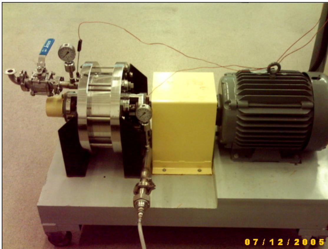
Fig. 3.2 - 12 HP Shockwave Power™ Reactor (10'' x 2'' pilot scale unit) (Reproduced with permission from Hydrodynamics Inc. Rome, GA).
