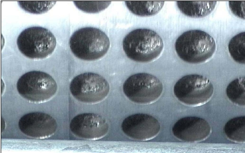
Fig.4.4 - Hydrodynamic cavitation within inner rotor cavities (Reproduced with permission from Hydrodynamics Inc. Rome, GA).
