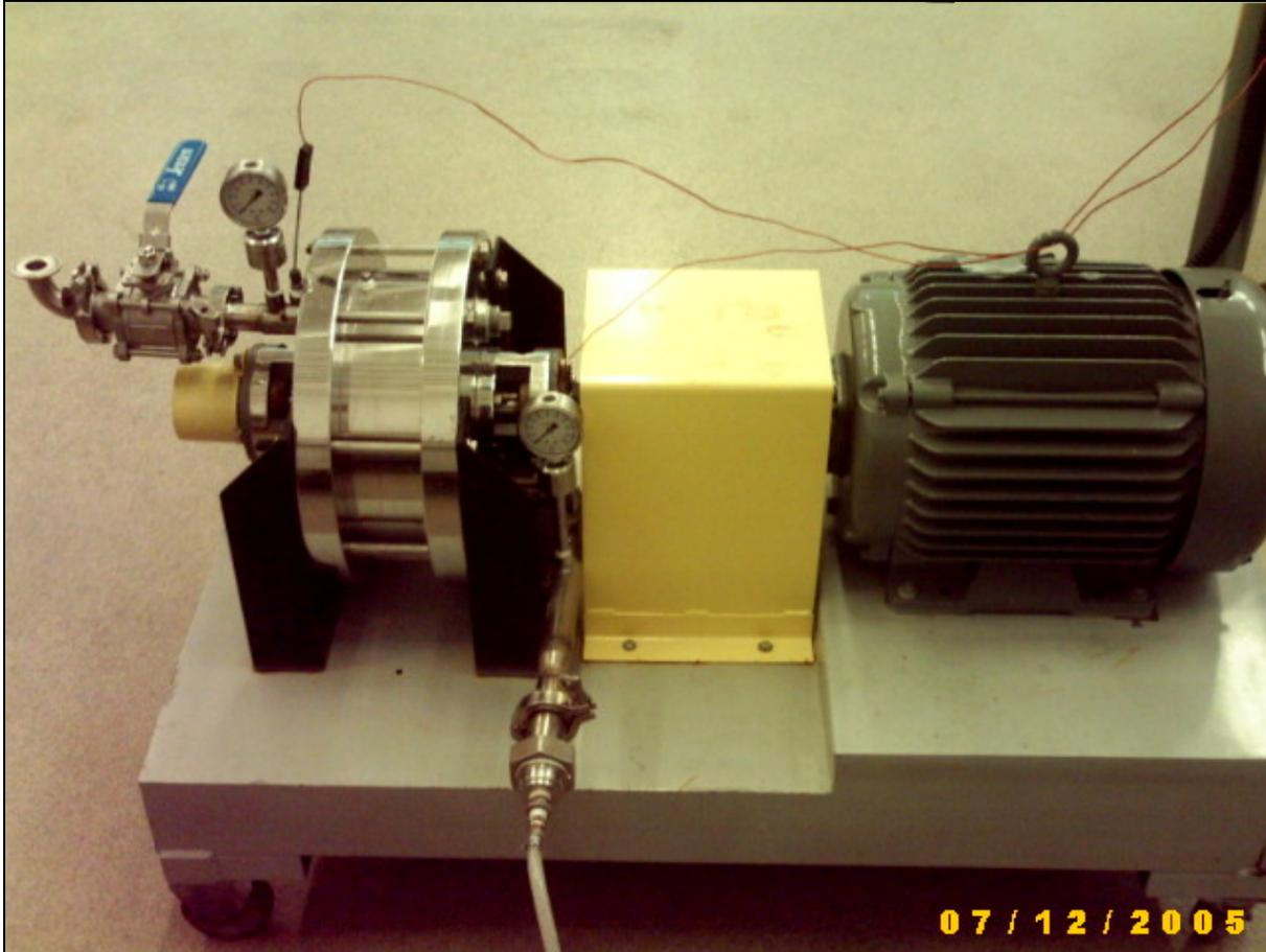
Fig. 2.2 -12 HP Shockwave Power™ Reactor (10" x 2" pilot scale unit) (Reproduced with permission from Hydrodynamics Inc. Rome, GA).
