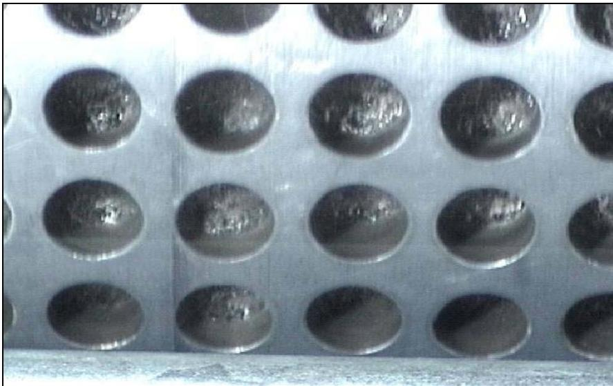
Fig. 1.6 - Hydrodynamic cavitation within inner rotor cavities (Reproduced with permission from Hydrodynamics Inc. Rome, GA).
