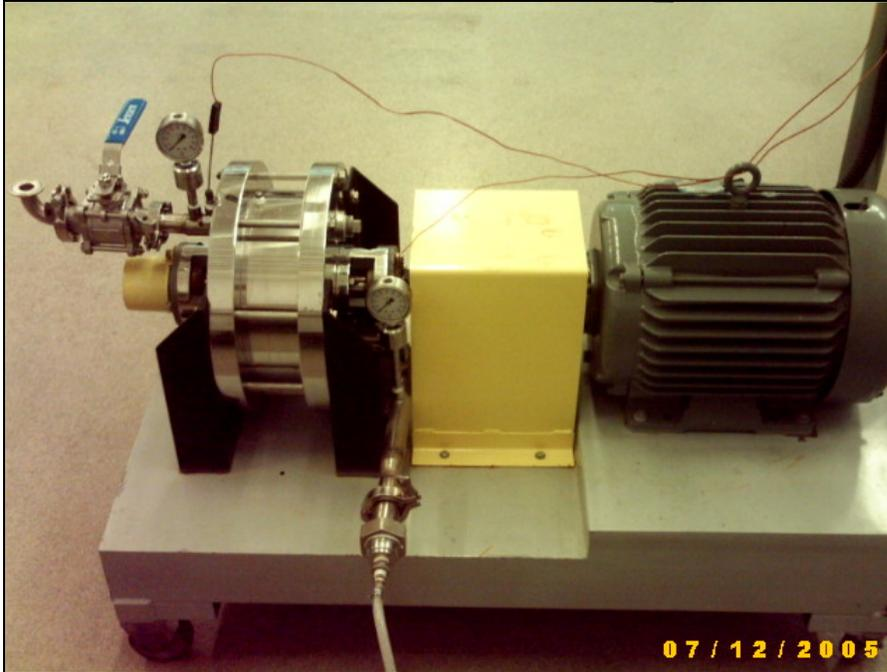
Fig. 1.5 - 12 HP Shockwave Power™ Reactor (10" x 2" pilot scale unit) (Reproduced with permission from Hydrodynamics Inc. Rome, GA).
