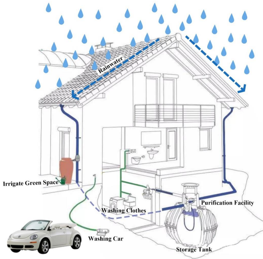
Figure 20: Roof rainwater harvesting system (enhanced by author)
