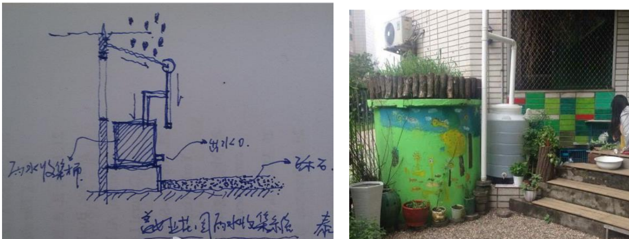
Figure 5: Rainwater harvesting system built in the yard
