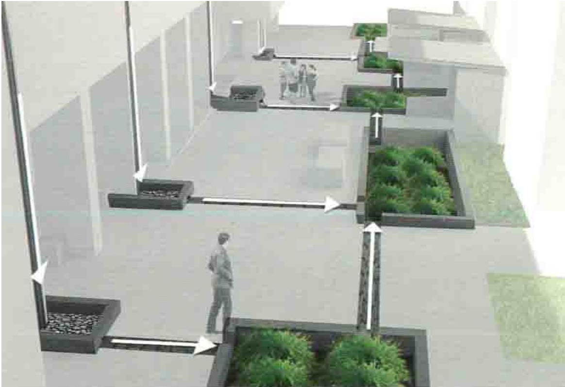
Figure 37: Perspective diagram of the stormwater management system in Stephen Epler Hall (Echols and Pennypacker 2015)
