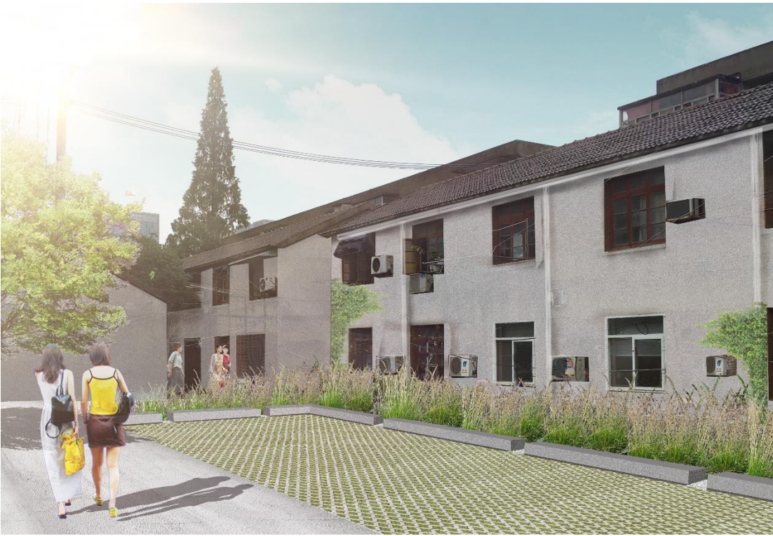
Figure 83: Pervious parking and bioretention planters (produced by author)
