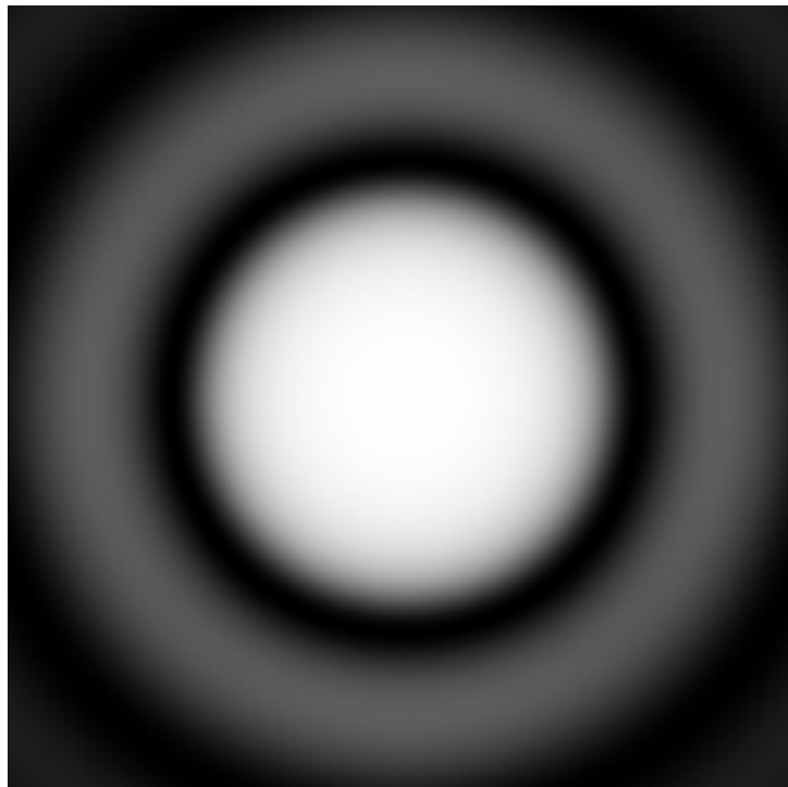
Figure 4b: Shape of Airy's disc as formed by the retinal light distribution due to diffraction.
