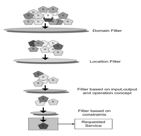
Figure 12: Filters in METEOR-S Semantic Web Service Discovery
